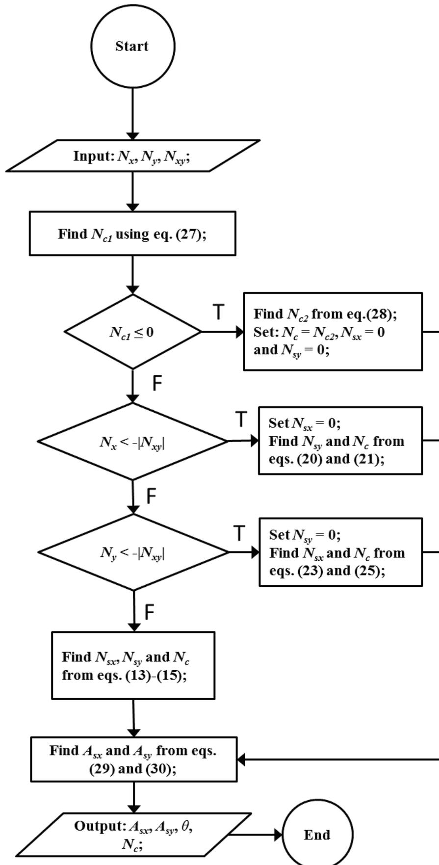
Algorithm 3 – Algorithm for finding real reinforcement force
