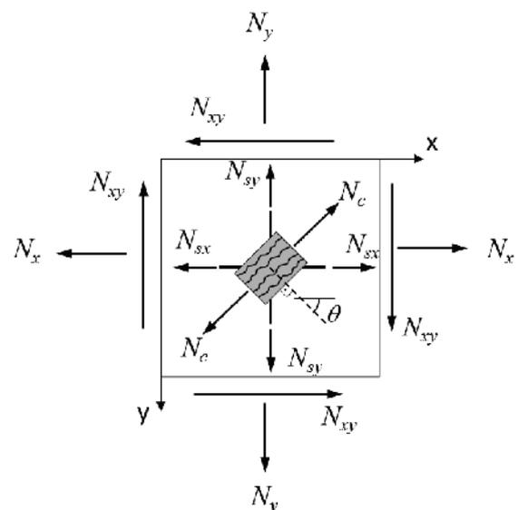
mechanical behavior of membrane elements with reinforcement in two orthogonal directions.
