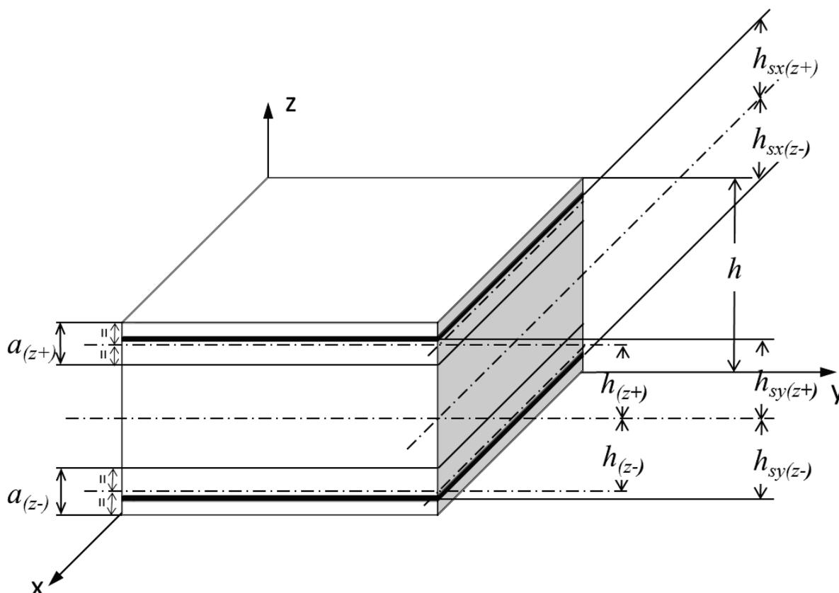
Figure 4 – Equilibrium conditions used to find the correct reinforcement force
