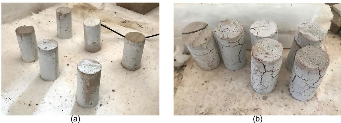
Figure 11. Bedding mortar specimens (a) one day after the test and (b) seven days after the test.
