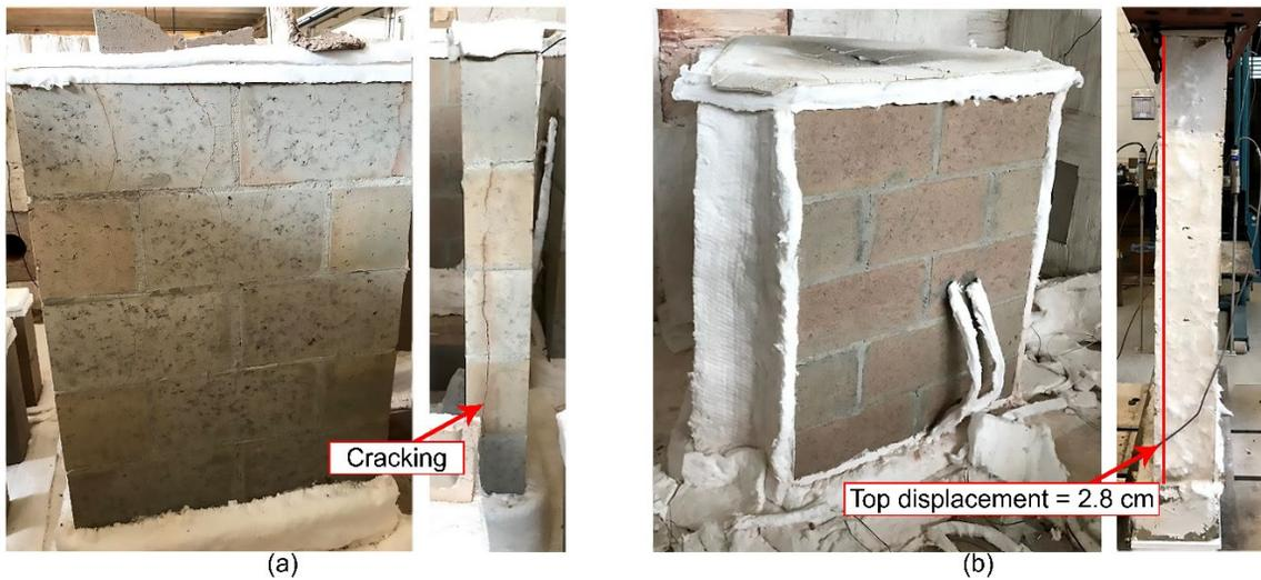
Figure 10. Small walls after the test: fire on (a) all faces and (b) one face (trio).
