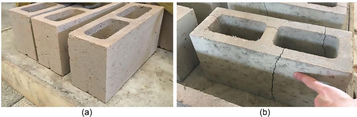
**Figure 9.** Blocks with nominal strength of (a) 4 MPa and (b) 10 MPa after heating.
