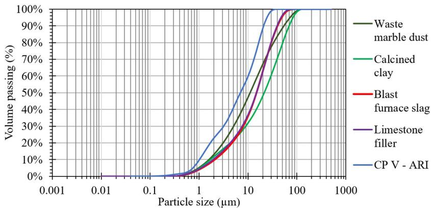
**Figure 1.** Particle size distribution of the waste marble dust, calcined clay, blast furnace slag, limestone filler and CP V-ARI cement.
