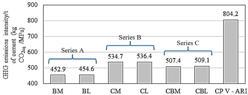
Figure 7. GHG emissions per tonne of blended cements and of CP V-ARI (in CO<sub>2eq</sub>).
