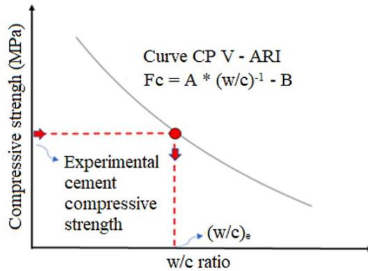
Figure 3. Method for obtaining the effective water/cement ratio ((w/c)<sub>e</sub>).
