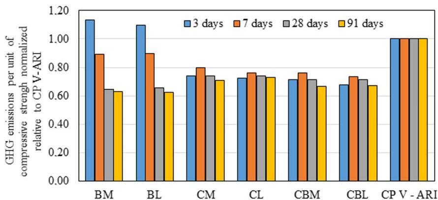
Figure 8. GHG emissions intensity per unit of compressive strength (CO<sub>2eq</sub>/MPa) of the studied cements at the ages of 3, 7, 28 and 91 days, normalized relatively to CP V-ARI.
