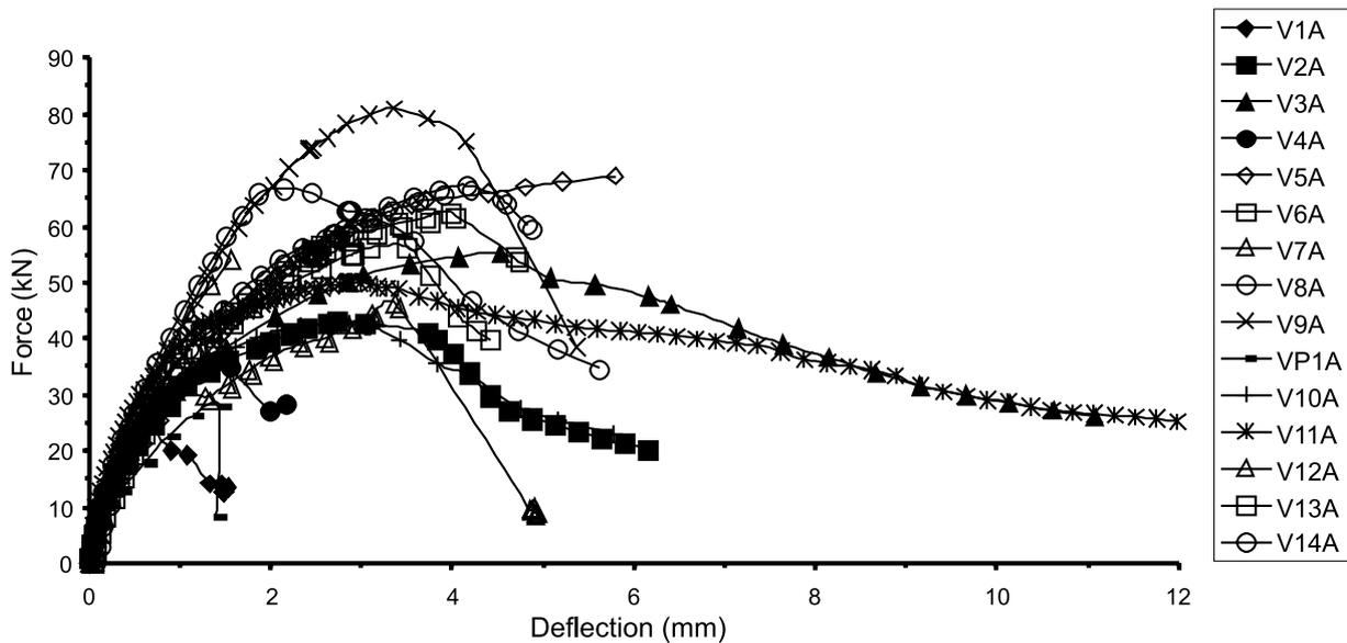
Figure 9 – Normalized load versus midpoint deflection for slabs
