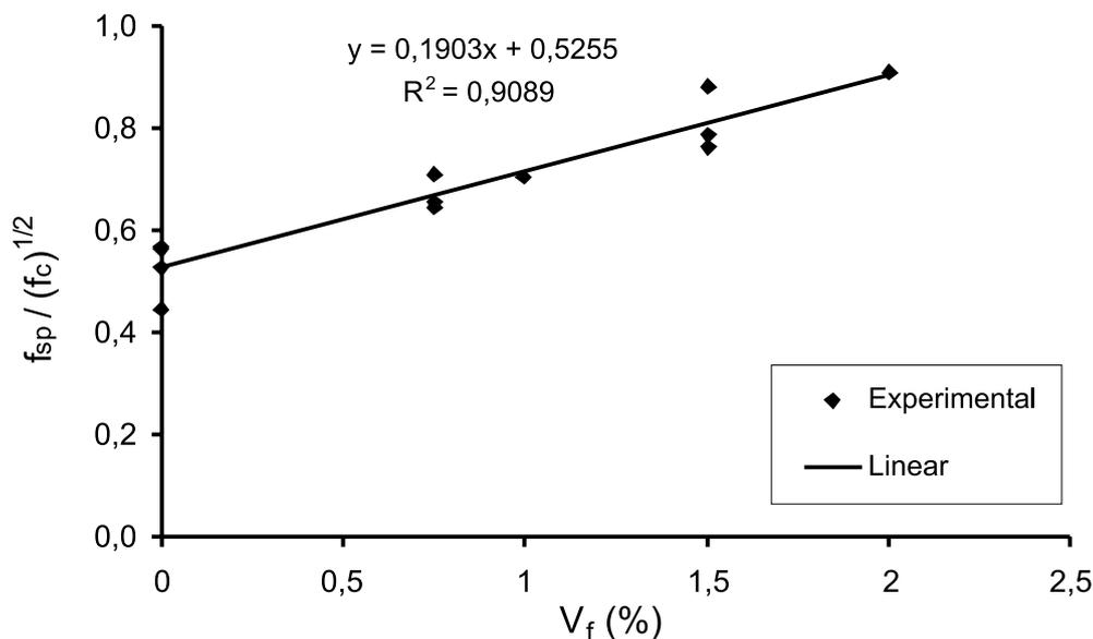
Figure 7 - Punching shear versus fiber volume fraction for slabs specimens
