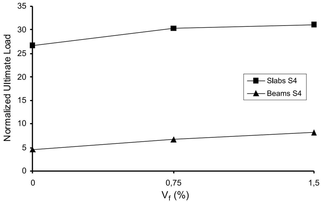
Figure 14 - Normalized ultimate load versus fiber volume fraction for specimens of Series 5
