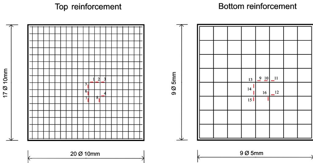
a) Location of the electric strain gages in steel reinforcement bars
