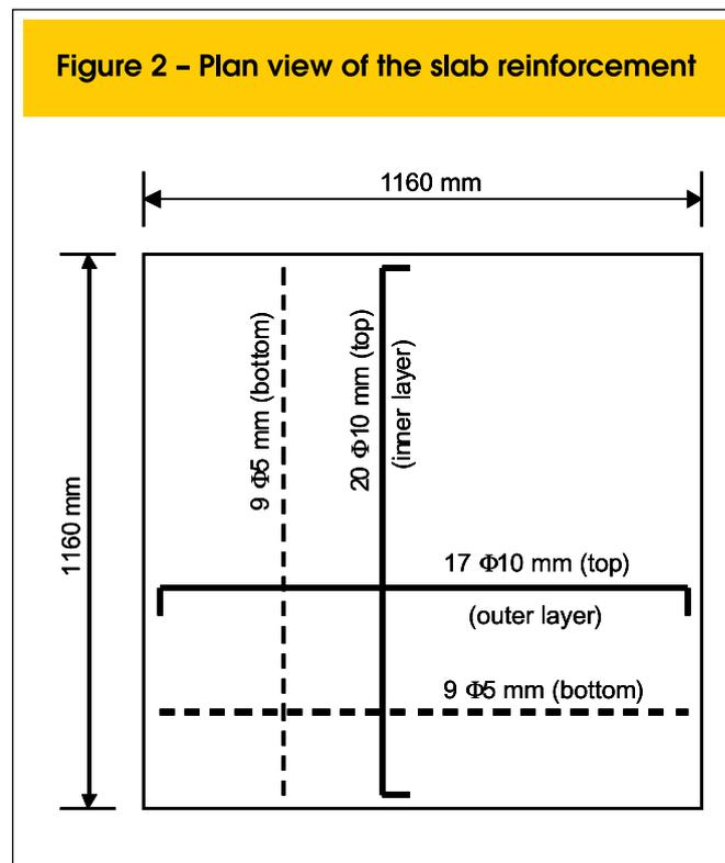
Figure 3 – Slab reinforcement details
