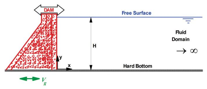
Figure 1 Scheme of the dam-reservoir interaction
