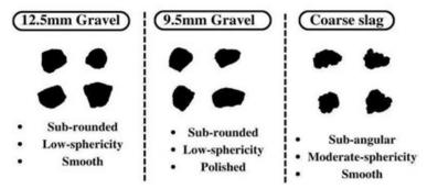
Figure 3. Digital Image Processing results for all coarse aggregates.
