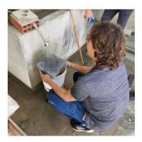
(b) Flow coefficient test.
