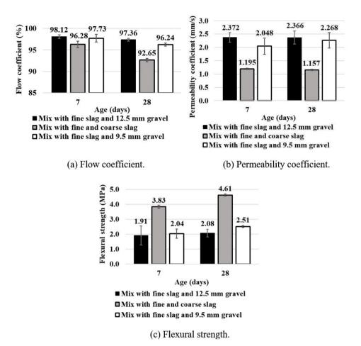
Figure 7. Result tests on concrete slabs.
