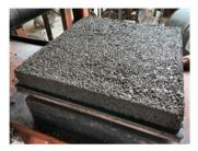
(c) Initial concrete slabs (50 cm×50 cm×6 cm).
