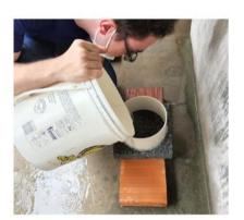
(a) Permeability coefficient test
