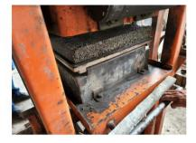
(b) Vibro-press machine in operation.
