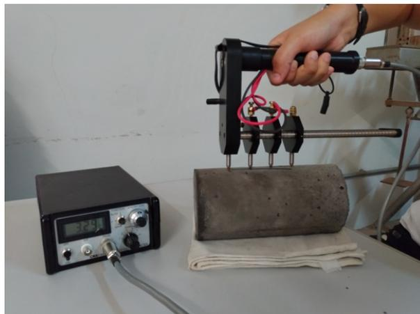
**Figure 1.** Surface electrical resistivity test by Wenner method in a cylindrical specimen.
