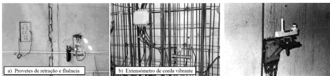
Figure 2. Instrumentation for the Rio-Niterói Bridge installed during its construction [18, p. 3].
