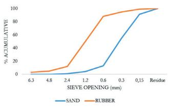
Figure 1 Granulometric curve of sand and rubber
