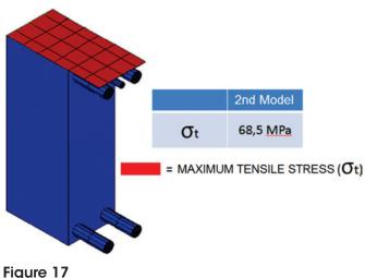
Stresses in the CFRP in the maximum momentum section
