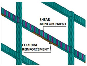
Figure 7 Positioning of reinforcement with CFRP – bottom view
