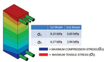
Figure 15 Stress in the concrete in the maximum momentum section
