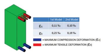
Figure 13 Deformation in the steel in the maximum momentum section
