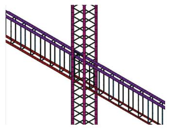
Figure 8 View of the reinforcement of the elements modeled on the beam-pillar connection
