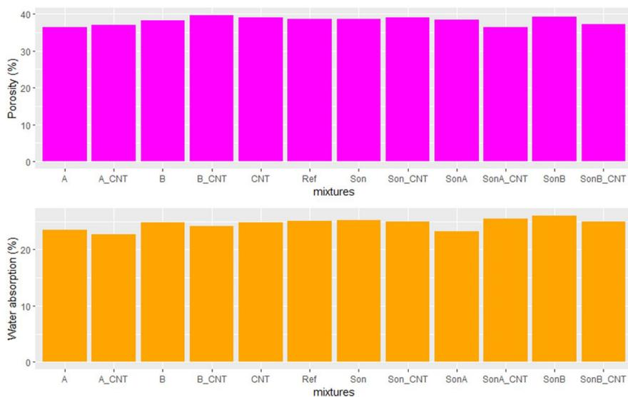
**Figure 13.** Porosity and water absorption of the hardened Portland cement pastes.
