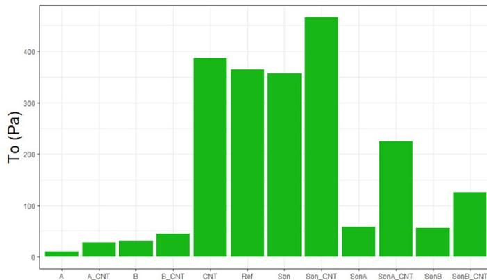
**Figure 7.** Static yield stress of the fresh Portland cement pastes.
