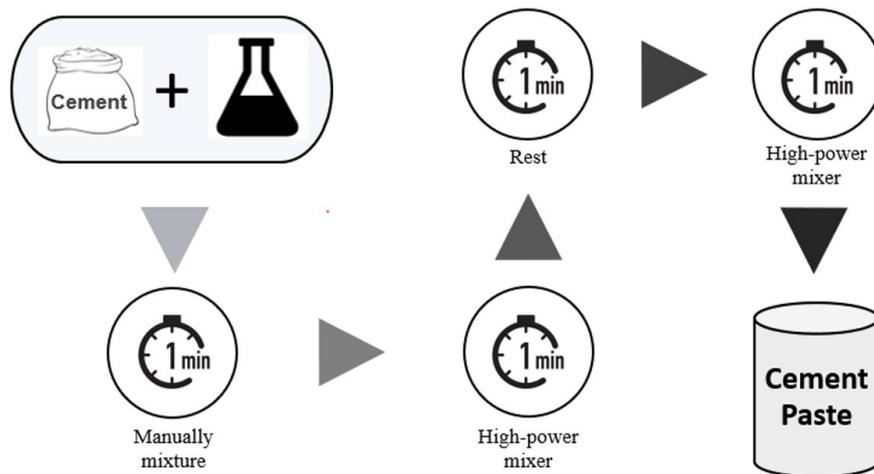
Figure 4. Cement pastes mixing procedure.
