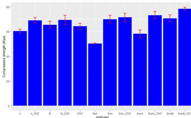
Figure 10. Compressive strength of the hardened Portland cement pastes.
