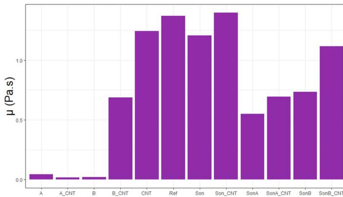
**Figure 9.** Apparent viscosity of the fresh Portland cement pastes.
