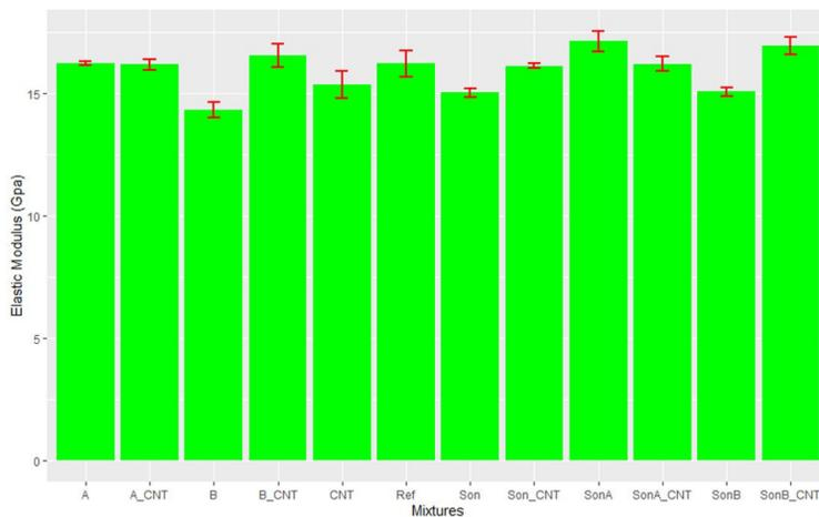
**Figure 11.** Elastic modulus of the hardened Portland cement pastes.
