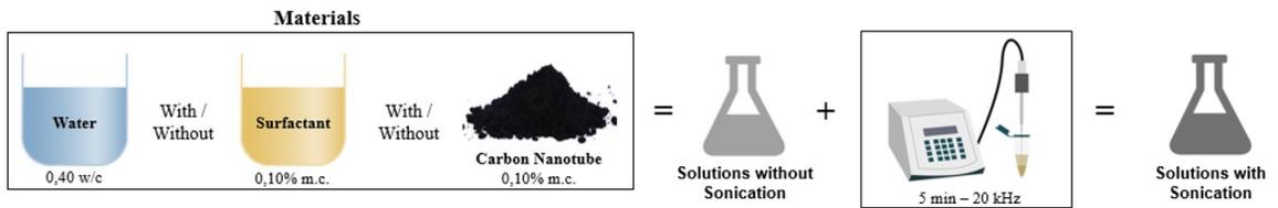
Figure 3. Preparation of solutions containing water, surfactants, and carbon nanotubes with and without the application of ultrasonication.
