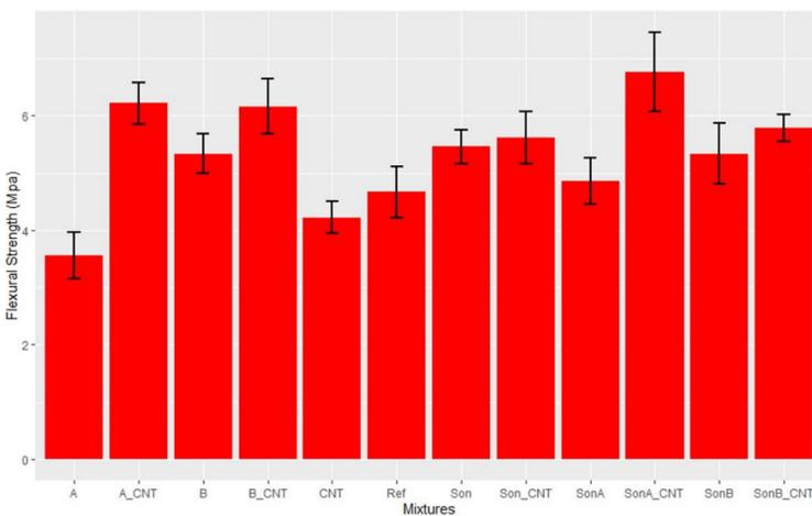
**Figure 12.** Flexural strength of the hardened Portland cement pastes.
