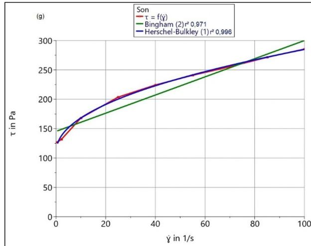
Figure 6. Rheological behavior curves of fresh Portland cement pastes fit with the Herschel-Bulkley and Bingham model.
