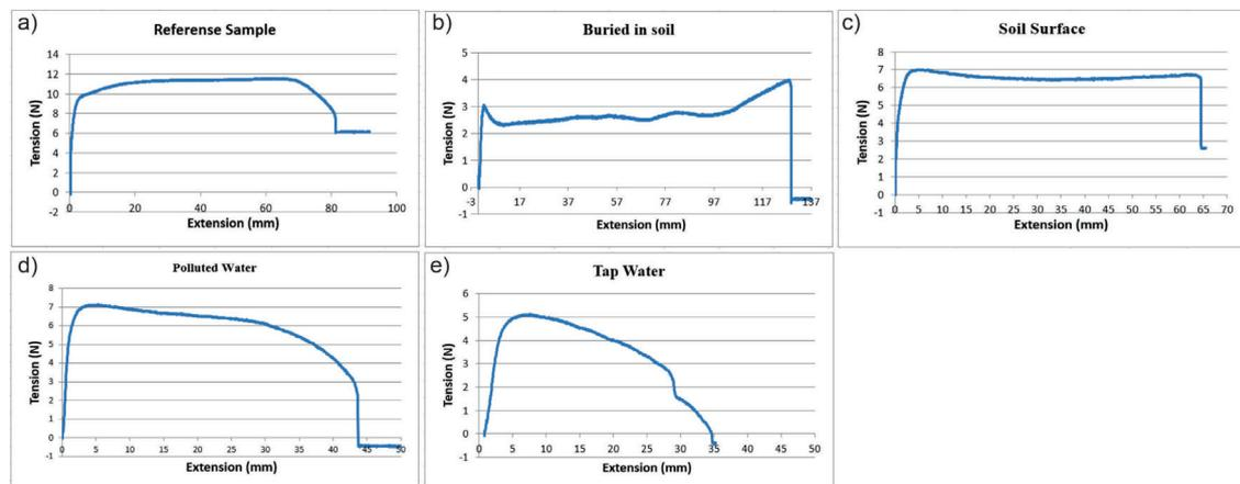
Figure 2: Tensile test for plastic bags: a) reference sample, b) buried in soil, c) exposed on soil surface, d) immersed in tap water, e) immersed in polluted water.
