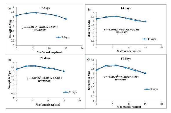
**Figure 5:** a) A trend of split tensile strength vs. % of rubber crumbs for 7 days curing spell, b) A trend of split tensile strength vs. % of rubber crumbs for 14 days curing spell, c) A trend of split tensile strength vs. % of rubber crumbs for 28 days curing spell, d) A trend of split tensile strength vs. % of rubber crumbs for 56 days curing spell.
