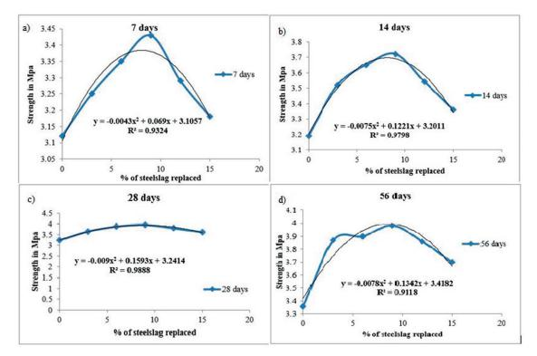
**Figure 6:** a) A trend of split tensile strength vs. % of steel slag for 7 days curing spell b) A trend of split tensile strength vs. % of steel slag for 14 days curing spell, c) A trend of split tensile strength vs. % of steel slag for 28 days curing spell, d) A trend of split tensile strength vs. % of steel slag for 56 days curing spell.
