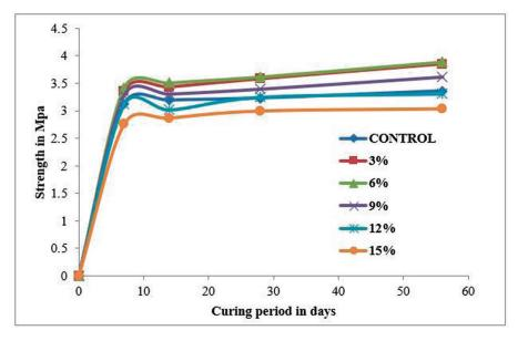
Figure 2: A family of curves (rubber crumbs against fine aggregate) for split tensile strength vs. curing spell in days.
