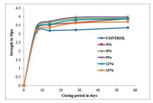
Figure 3: A family of curves (steel slag against cement) for split tensile strength vs. curing spell in days.
