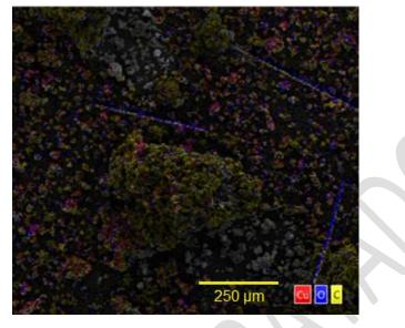
Figure 6: EDS mapping of Cu/XCTF sample.
