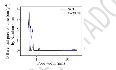
Figure 4: The pore size distribution, calculated from DFT (Density Functional Theory) method.
