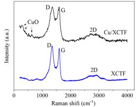
Figura 7: Raman spectra of the samples XCTF (A) and Cu/XCTF (B).
