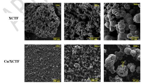
Figure 5: SEM-FEG images of XCTF and Cu/XCTF samples, at 250x, 850x and 5000x magnifications.
