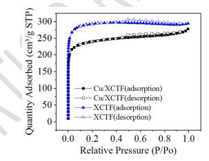
Figure 3: Nitrogen adsorption-desorption isotherms at 77 K (full and open symbols, respectively) of both samples.
