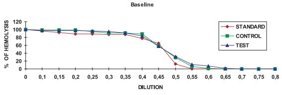
Figure 1 - Osmotic fragility - Curve of medium values of hemolysis of fresh blood collected in heparin (standard), stored in CPD-A1 with the compound WR6026 (Test) and without it (control) at baseline.
