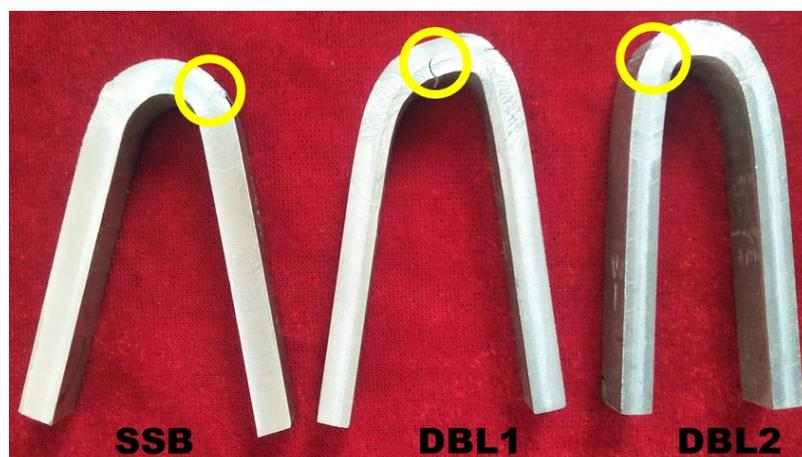
Figure 12. Macroscopic view of the root-bended welded sample
