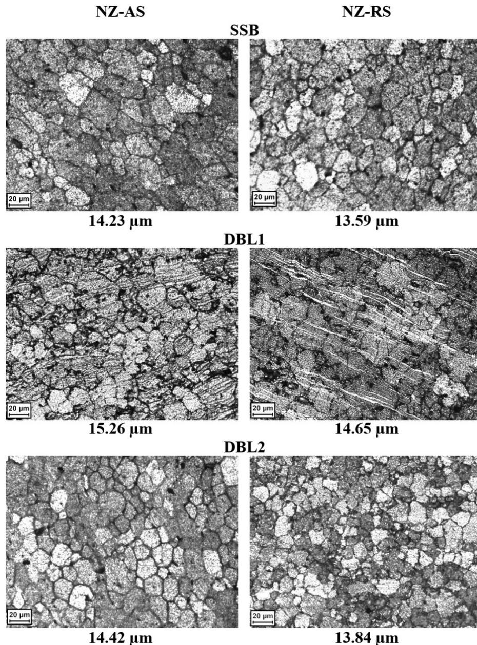
**Figure 9.** Metallographic images for the three different configurations in the advancing and retreating side of the NZ.
