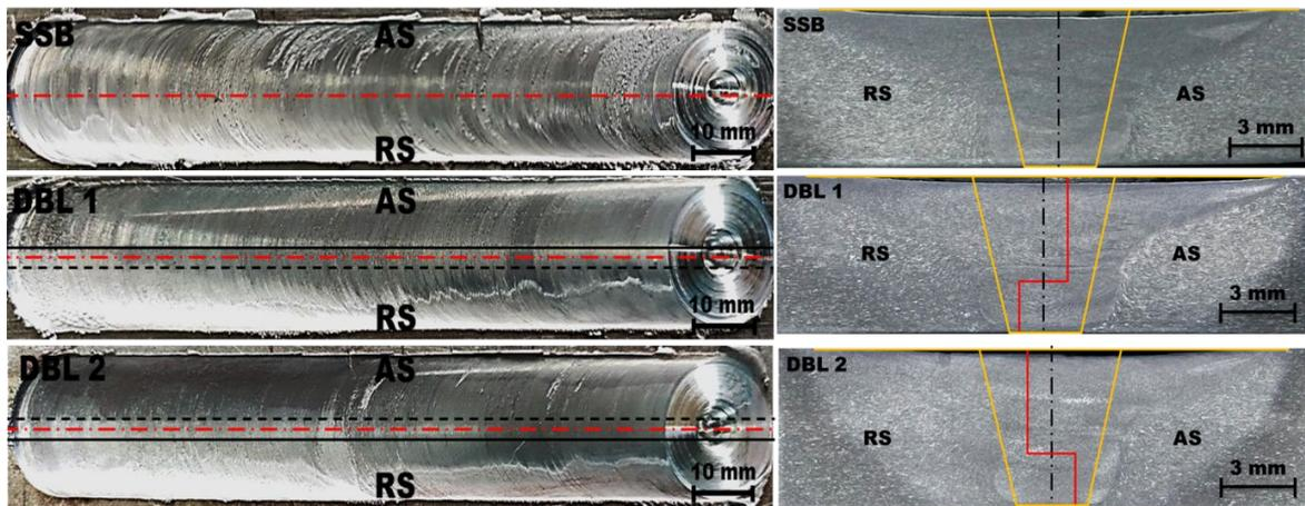
Figure 4. Weld bead appearance and respective macrostructure of joints formed with different joint line configuration.
