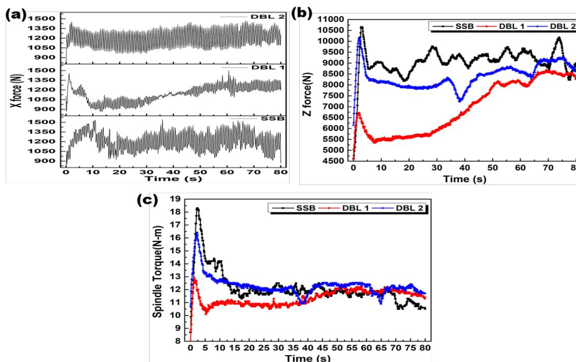
**Figure 3.** Comparison of force and torque of welding for different weld joint configuration, (a) Comparison of X-force; (b) Comparison of Z-force; (a) Comparison of spindle torque.
