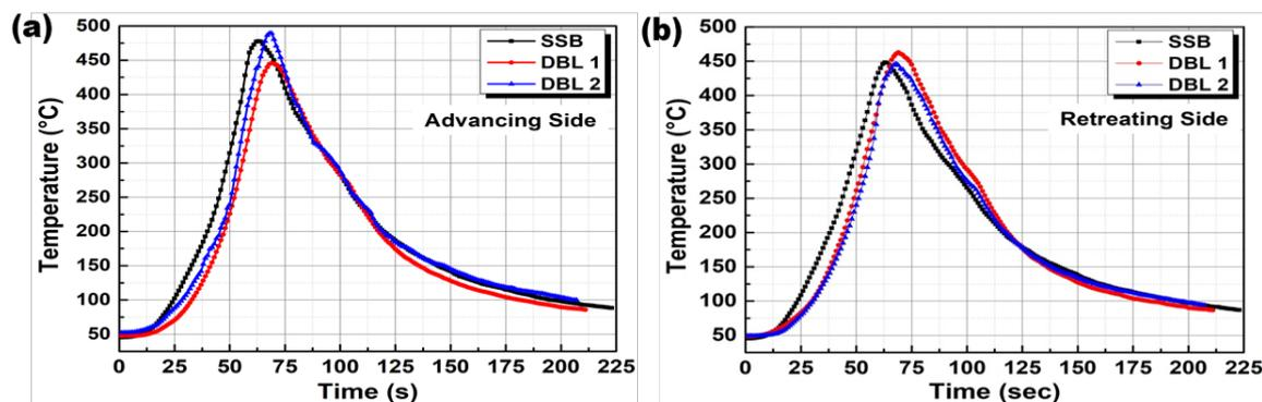
Figure 2. Weld thermal cycle for different joint configuration (a) Advancing side, (b) Retreating side.
