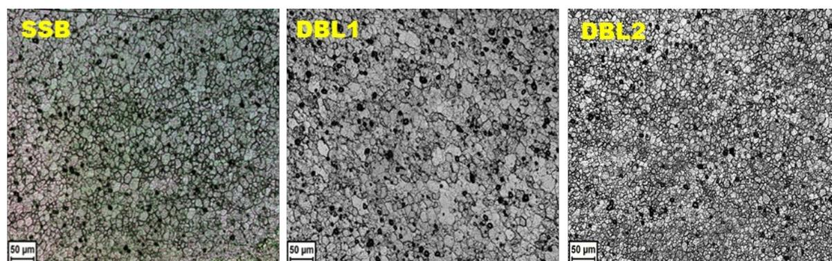
**Figure 8.** Metallographic images for the three different configurations in the middle of the NZ.
