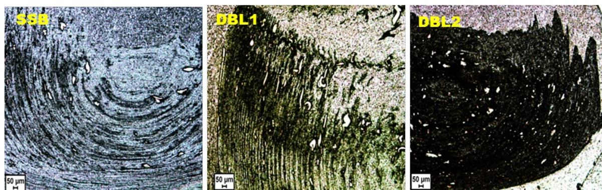
**Figure 7.** Metallographic observations for joint configuration showing the distribution and displacement of Cu particles.
