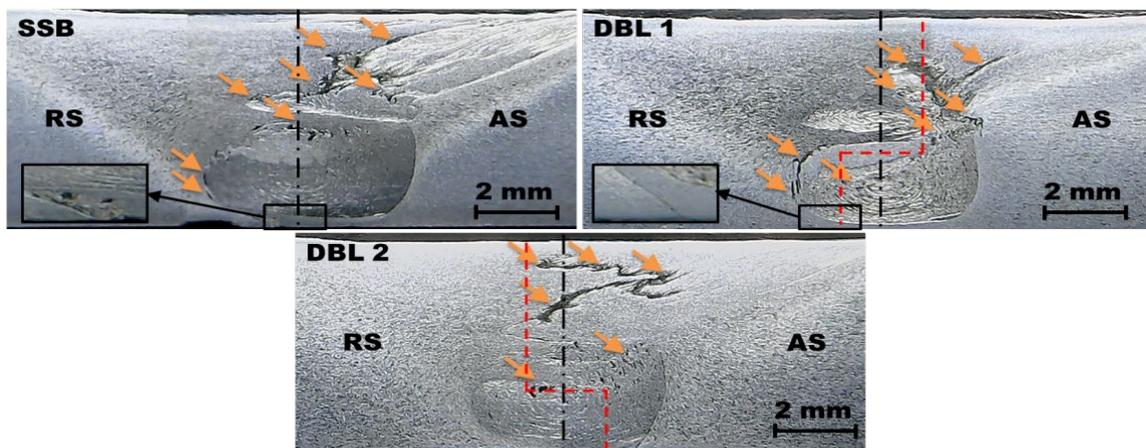
Figure 5. Macrostructure of the joints showing different types of material flow as an effect of variation in the joint configuration.
