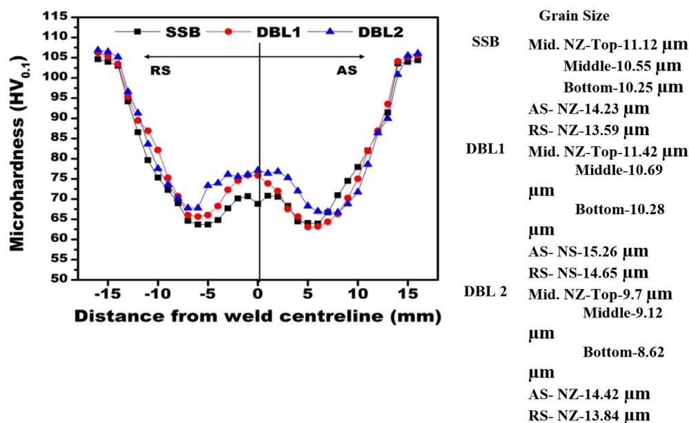
Figure 10. Microhardness distribution plot along the weld centreline for the three different joint configurations.
