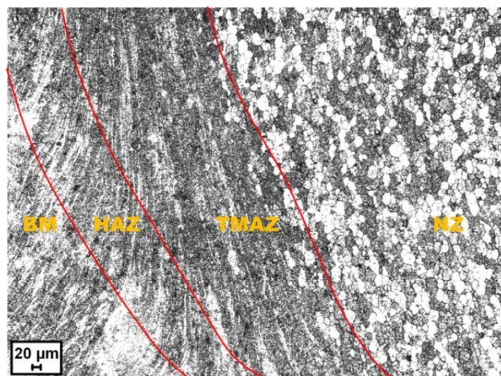
**Figure 6.** Typical zones of the SSB joint configuration.
