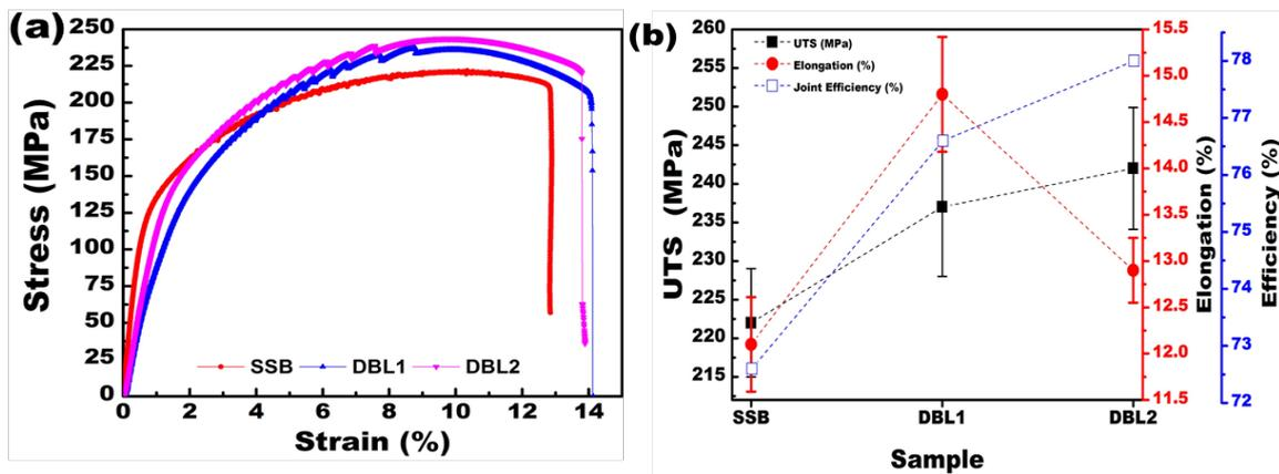
Figure 11. Comparison of the tensile strength, (a) comparison of the tensile plot for different types of welding and (b) Comparison of UTS, % Elongation and joint efficiency of different DBL configured welded joint with SSB configured welded sample.
