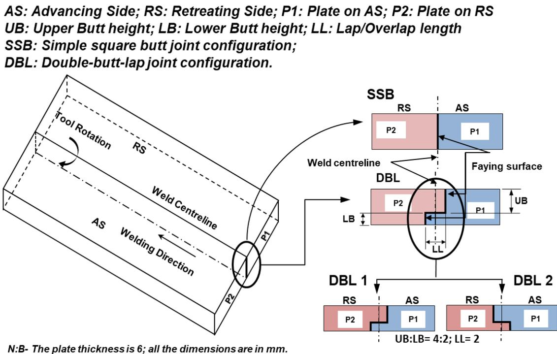
Figure 1. Schematic representation of SSB and DBL joint configuration.
