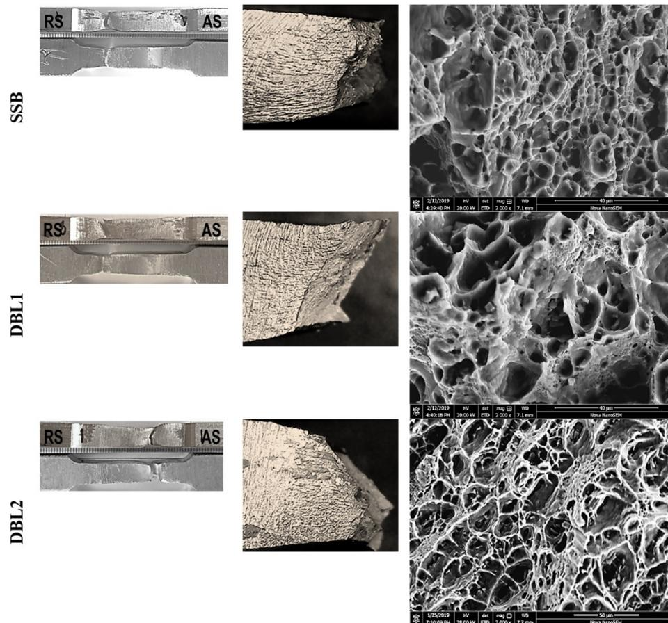
**Figure 13.** Fracture analysis of tensile fractured samples showing the different views of tensile fractured samples, close view of the fractured sample and the respective fractography.
