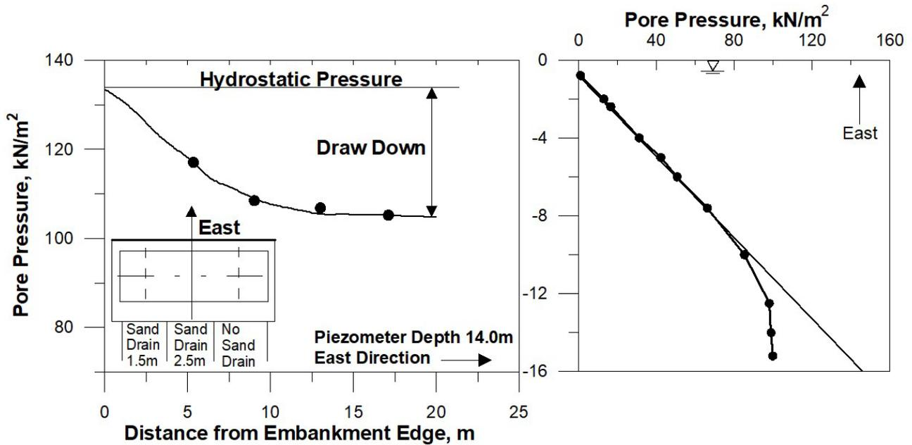
Figure 5. Piezometric pressure vs. distance from the edge of the embankment at RTN Dockyard site (East direction).
