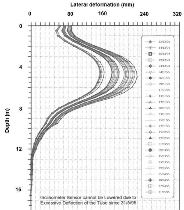
Figure 21. Lateral deformation with depth below embankment TS3 at the SBIA site in Bangkok.
