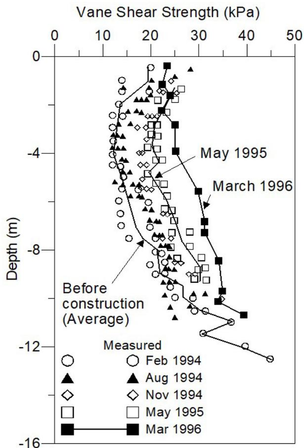
**Figure 31.** Field vane shear strength as measured in embankment TS3 at SBIA site.
