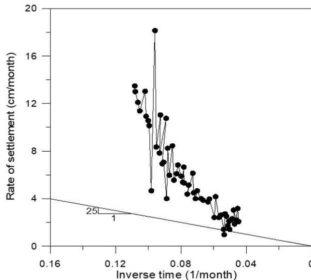
Figure 28. Rate of settlement versus inverse time plot at SBIA site.
