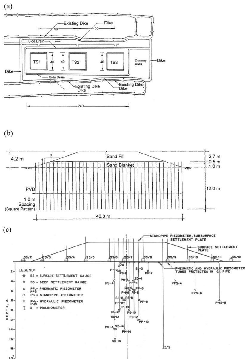
**Figure 19.** (a) site plan of test embankments TS1, TS2 and TS3 at SBIA site; (b) test section TS3 showing PVD at SBIA site; (c) section view of the test embankment showing the position of instruments at the Second Bangkok International Airport (SBIA).
