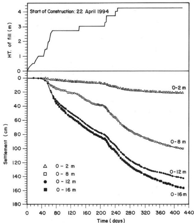
Figure 20. Settlement-time plot of the embankment with PVD at the SBIA site in Bangkok.
