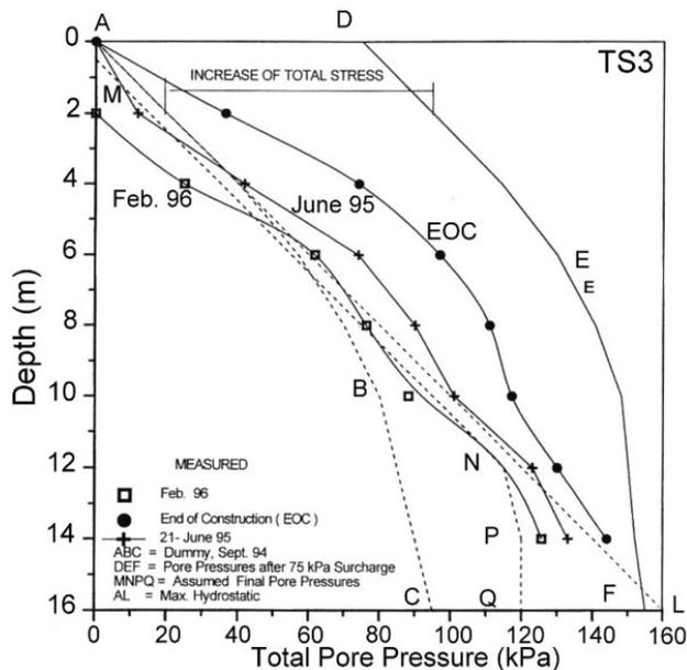
Figure 26. Pore pressure profile of test embankment with PVD at SBIA site.
