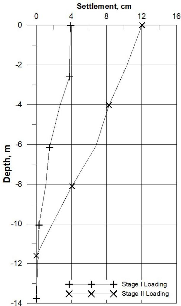
Figure 7. Immediate settlement below embankment at RTN Dockyard site.
