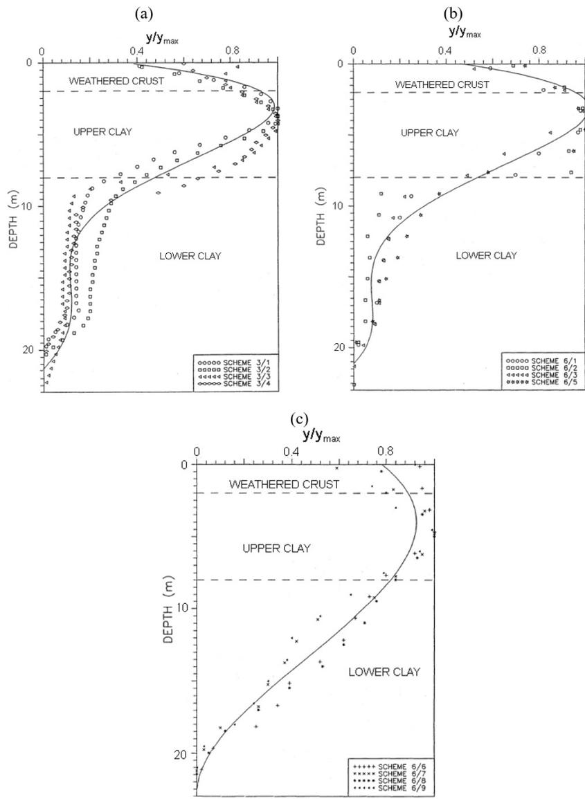
**Figure 14.** Variation of ratio of lateral deformation to maximum lateral deformation with depth for (a) 3 m-high embankments, (b) and (c) 6 m-high embankments.
