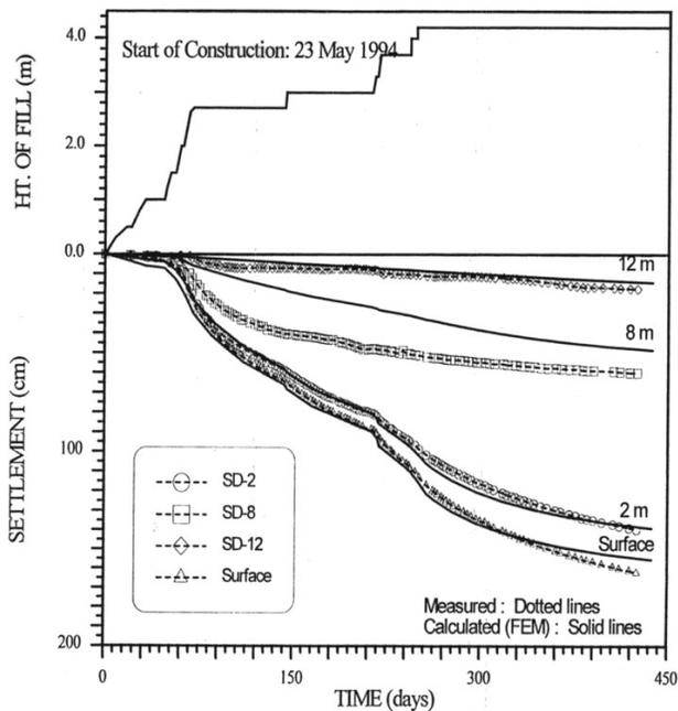
Figure 23. Measured and computed settlement with different depth at the SBIA site in Bangkok.
