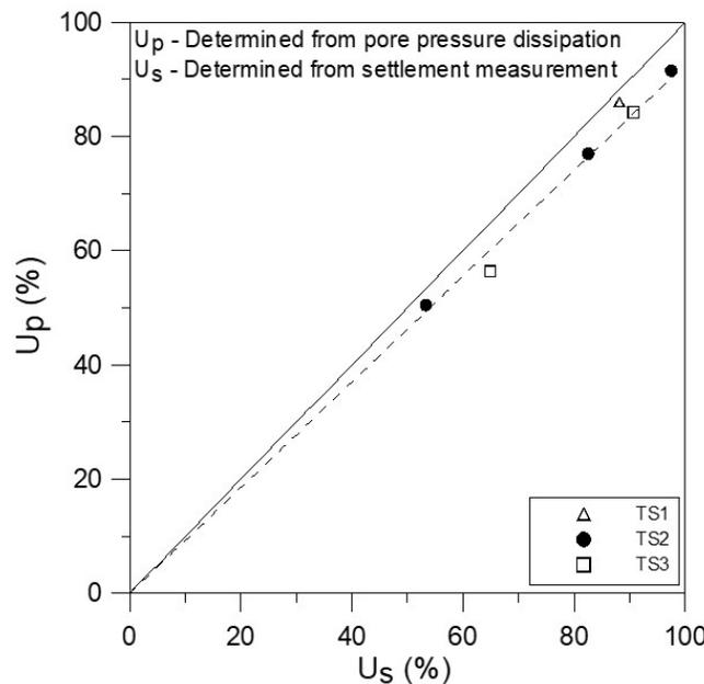
Figure 27. Degree of consolidation computed from pore pressure dissipation and settlement measurements at SBIA site.
