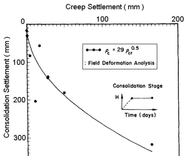
Figure 17. Variation of consolidation settlement with respect to creep settlement.
