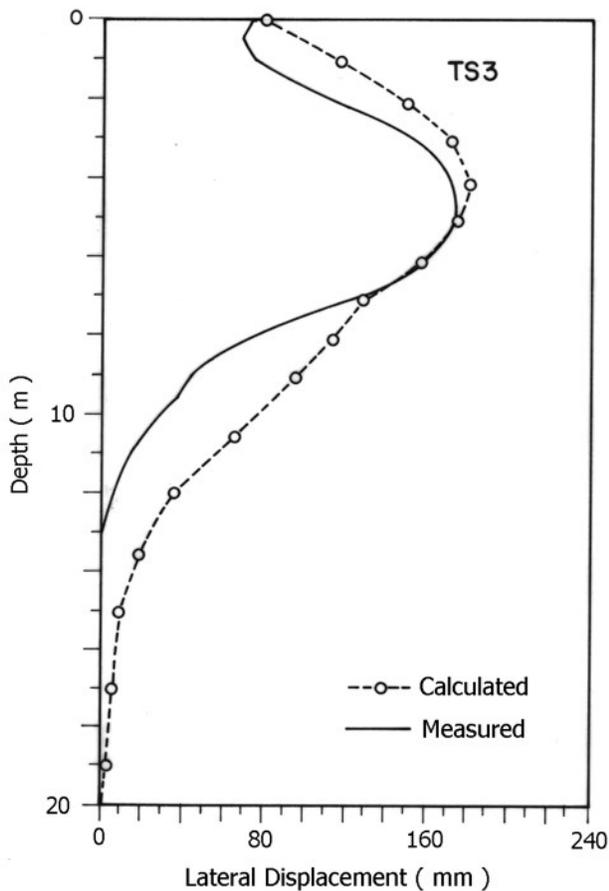
Figure 24. Measured and computed lateral movement of the embankment at the SBIA site in Bangkok.
