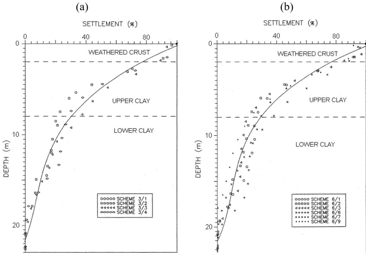
**Figure 12.** (a) variation of percentage settlement with depth for 3 m high dmbankments; (b) variation of percentage settlement with embankments depth for 6 m high.
