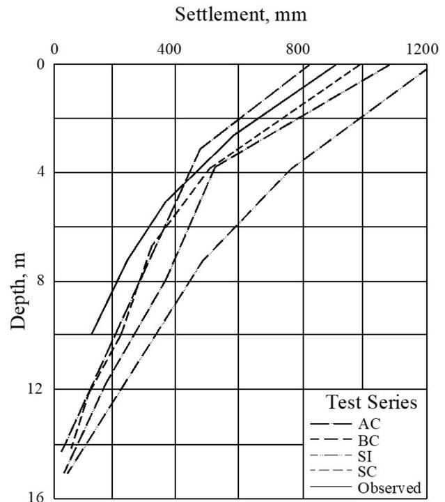
Figure 8. Consolidation settlement below embankment as calculated at RTN Dockyard site.
