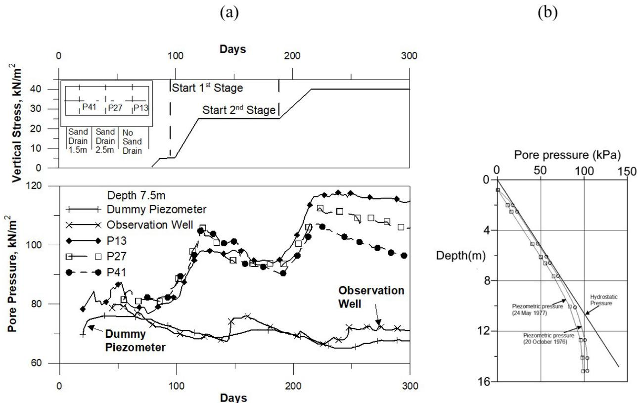
Figure 4. (a) typical piezometer readings at RTN Dockyard site; (b) variation of piezometric pressures with depth at RTN Dockyard site.
