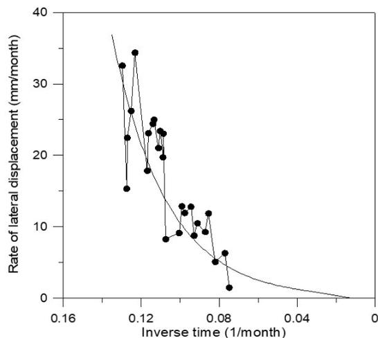
**Figure 29.** Rate of lateral movement versus inverse time plot at SBIA site.
