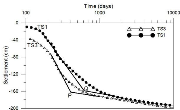
**Figure 30.** Settlements versus log-time plot for embankments TS1 and TS3 at SBIA site.
