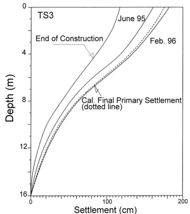
Figure 22. Settlement plot of test embankment with PVD at SBIA site.
