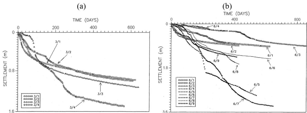
**Figure 13.** (a) comparison of maximum settlement profiles with time for 3 m-high embankments; (b) comparison of maximum settlement profiles with time for 6 m-high embankments.
