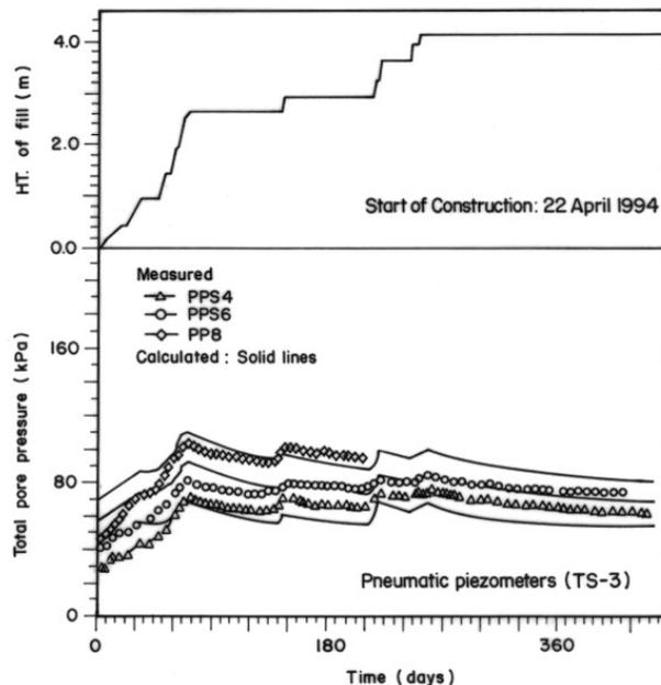
Figure 25. Measured and computed pore pressure dissipation of the embankment at the SBIA site in Bangkok.
