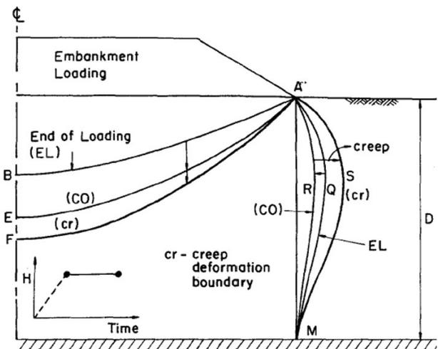
Figure 11. Deformation pattern of embankment foundation at end of consolidation stage.
