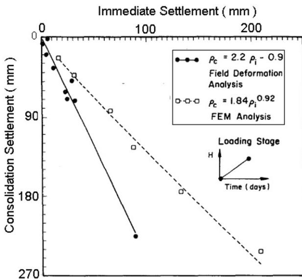
Figure 16. Variation of consolidation settlement with respect to immediate settlement.
