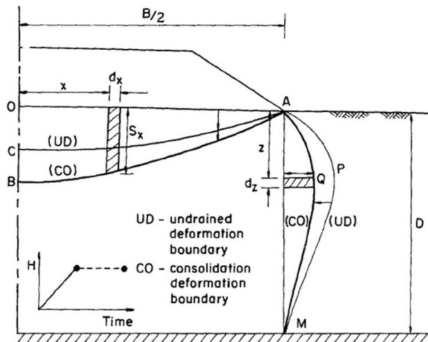
Figure 10. Deformation pattern of embankment foundation at end of loading stage.
