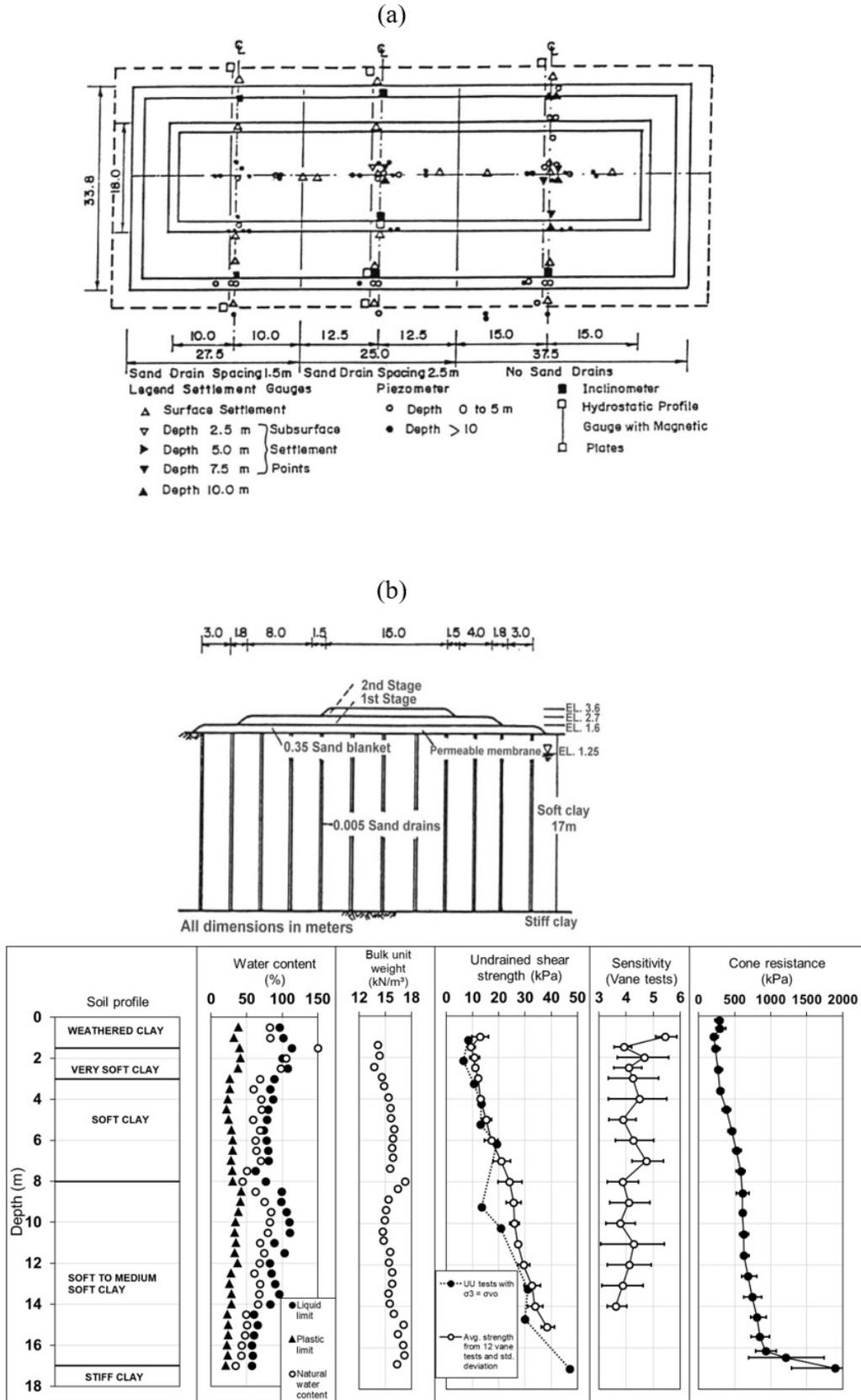
Figure 2. (a) plan of test embankment at RTN Dockyard site; (b) elevation of test embankment at RTN Dockyard site; (c) general properties of Pom Prachul Clay at RTN Dockyard site.
