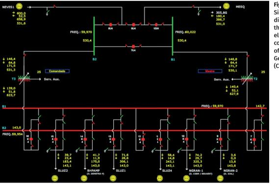
Figure 1. Single-line diagram of the energy electric company of Minas Gerais (CEMIG). being considered high in a scale between 0 and 17 related to the impact that it could cause.
