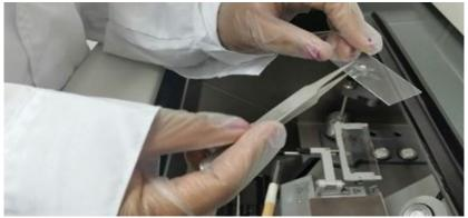
Figure 2. Removing tapes from the Leica CM 1520 cryostat for the preparation of slides for viewing the cortex by optical microscopy.
