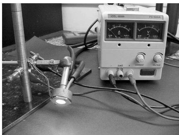
Figure 3 - LED-based device emitting red light at an emission peak at 626 nm.
