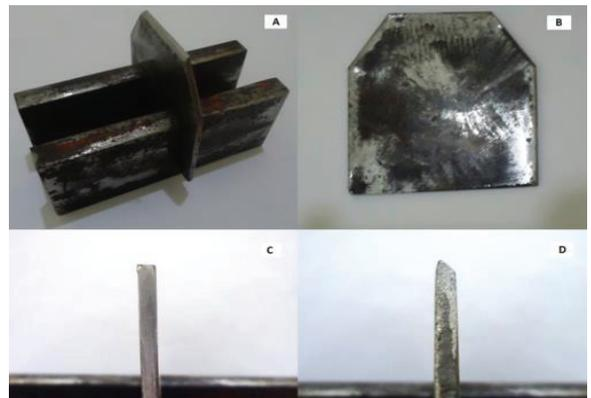
**Figure 5.** Apparatus developed for the shear test (A), blade used for test (B), without tensioner (C), and blade with tensioner and 45° chamfer at the end (D).
