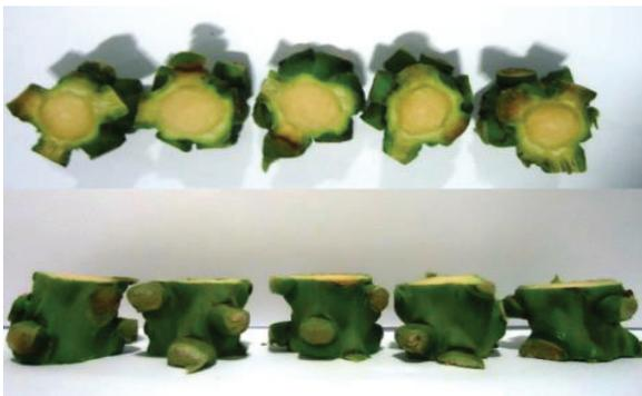
**Figure 6.** Test specimens of macaw palm rachis prepared for compression tests.
