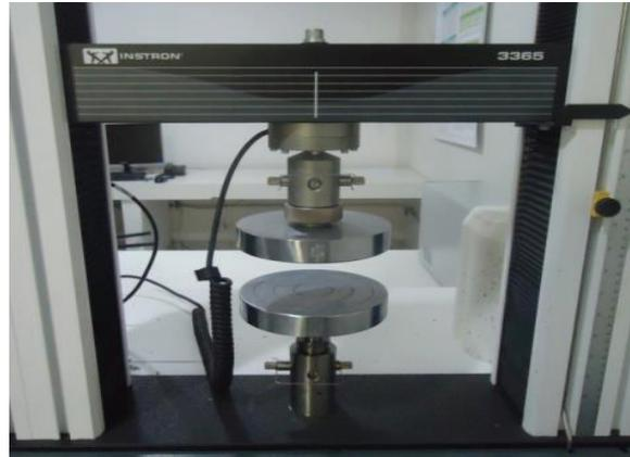
**Figure 7.** Equipment used for compression test of macaw palm rachis.
