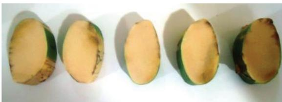
**Figure 3.** Test specimens of macaw palm rachis prepared for shear test.
