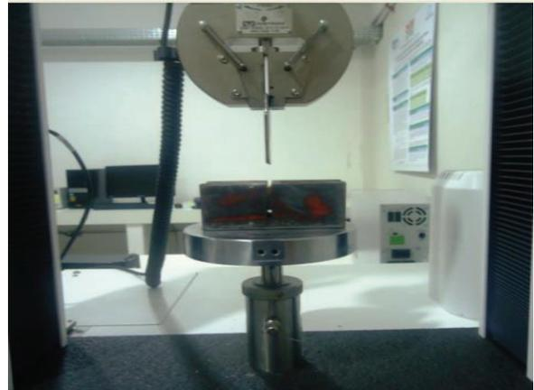
**Figure 4.** Set up used for the shear test of macaw palm rachis.
