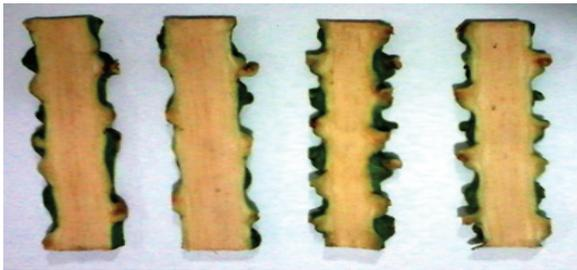
**Figure 2.** Test specimens of macaw palm rachis used to determine the Poisson's ratio.
