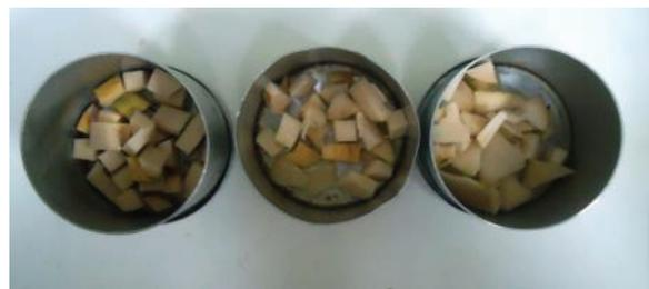
**Figure 1.** Crucibles containing chopped samples of macaw palm rachis with a volume of 1 cm<sup>3</sup>.
