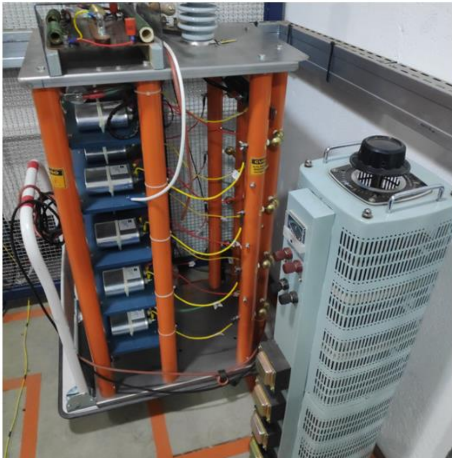
Figure 8. Laboratory portable impulse current waveform low energy.
