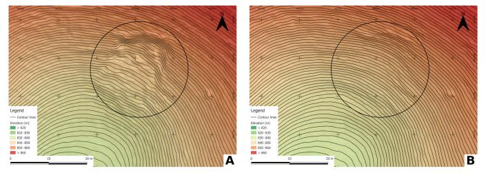
**Figure 2:** Reconstruction of topography for volume calculation. A) Contour lines deformed by the slide event; B) Contour lines reconstruction. Example from the TLS point cloud DEM with 50 cm spatial resolution and contour lines with 50 cm interval.
