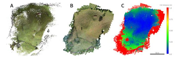
Figure 3: A) TLS point cloud; B) SfM-MVS point cloud; C) Cloud-to-Cloud distance with 1 m threshold using the TLS as the reference cloud.
