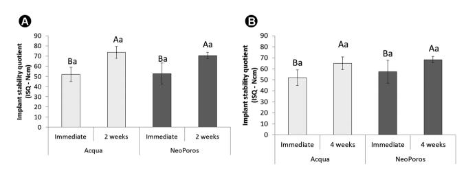
Figure 1. A: Implant stability quotient values for 2 weeks. Different letters represent significant difference, uppercase letter for periods of evaluation and lower case letters for implant type comparison; B: Implant stability quotient values for 4 weeks. Different letters represent significant difference, uppercase letter for periods of evaluation and lower case letters for implant type comparison.
