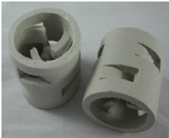
Figure 2: Ceramic Pall Ring packing used in this research.
