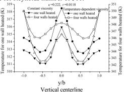
Figure 7: Temperature distributions at the vertical centerline.
