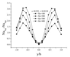
**Figure 11:** Distribution of Nu<sub>lvp</sub> - Nu<sub>lcp</sub> along the inner heated wall for different Reynolds number
