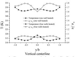
**Figure 9:** Temperature and viscosity distributions at the vertical centerline for temperature-dependent viscosity.
