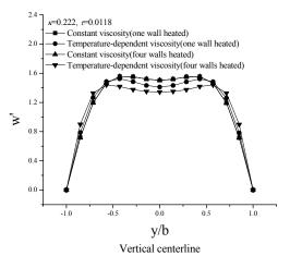
**Figure 5:** Axial velocities at the vertical centerline for Reynolds number of 300.
