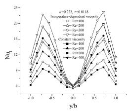
**Figure 10:** Distribution of local Nusselt number along the inner heated wall for different Reynolds number.
