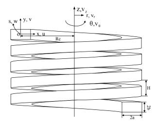
Figure 1: Schematic geometry and coordinates of the helical rectangular duct model.
