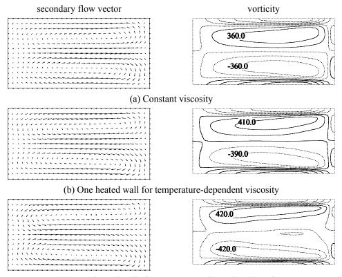
(c) Four heated walls for temperature-dependent viscosity
