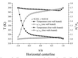
**Figure 8:** Temperature and viscosity distributions at the horizontal centerline for temperature-dependent viscosity.
