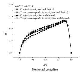
**Figure 4:** Axial velocities at the horizontal centerline for Reynolds number of 300.
