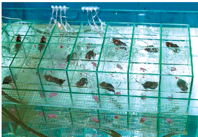
Figure 1. Swimming apparatus for mouse physical training.
