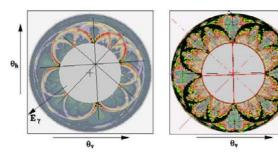
Figure 2. (Left) Simulated scan illustrating the alignment procedure by fitting a template. Here the face of the crystal, i.e. the [100] plane, is offset in  $\theta_{\rm v}$  and  $\theta_{\rm h}$  with respect to the direction of the incident electron beam. (Right) Final scan taken during a data scan run. We see that the crystal is aligned to the desired degree of precision.
