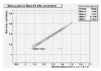
Figure 8. The relative kinematics of the  $K^+$  and  $p+\pi^-$  components of the overall reaction.
