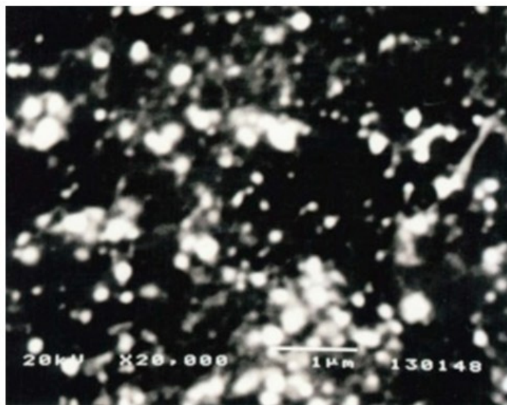
FIGURE 3 - SEM image of gold coated Fe 3 O 4 particles (N).
