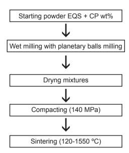
Figure 1: Schematic diagram showing the main steps of the process, used in this work.
