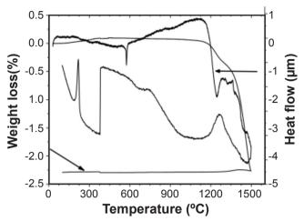
Figure 7: DTA and TG curves of samples containing 30 wt.% CP. [Figure 7: Curvas ATD e TG das amostras contendo 30% peso CP.]
