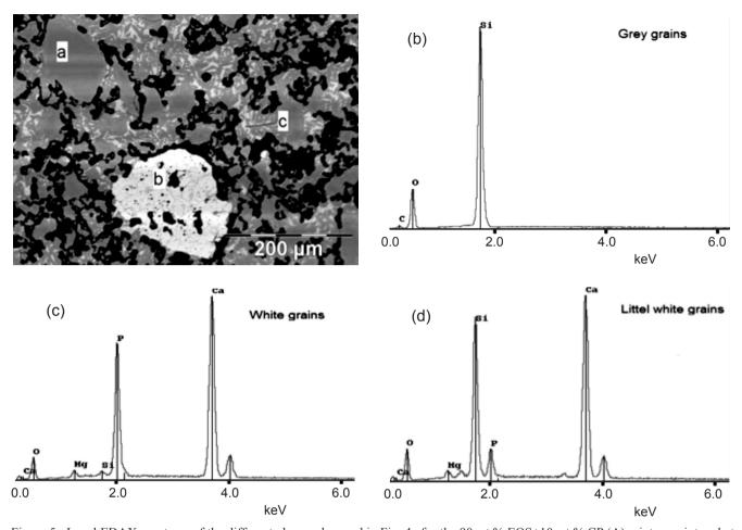
Figure 5: Local EDAX spectrum of the different phases observed in Fig. 4a for the 90 wt.% EQS+10 wt.% CP (A) mixtures sintered at 1300 °C for 4 h, (B) grey grains (a), (C) white grains (b), and (D) small white grains (c). [Figura 5: Espectro EDX das differentes fases observadas na Fig. 4a para 90% peso EQS + 10% peso CP (A) misturas sinterizadas a 1300 °C por 4 h, (B) grãos cinza (a), (C) grãos brancos (b), e (D) pequenos grãos brancos (c).]
