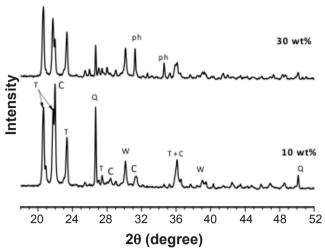
Figure 3: XRD patterns of samples of EQS with different CP additions sintered at 1300 °C for 4 h. Q (quartz); C (cristobalite); T (tridymite); W (wollastonite); ph (phosphate mineral).
