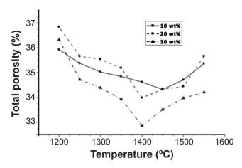
Figure 8: Total porosity of the samples with different CP additions, sintered at different temperatures for 2 h.
