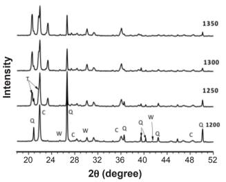
Figure 2: XRD patterns of samples of EQS + 10 wt% CP sintered at various temperatures for 2 h. Q (quartz); C (cristobalite); T (tridymite); W (wollastonite)...
