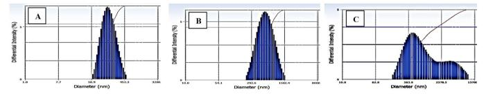
Figure 4. Particle size distributions for spray-dried nanocapsules coated with different secondary coating materials. A. 10% maltodextrin (MD, DE 18), B. 10% whey protein concentrates (WPC), C. 10% arabic gum (AG).
