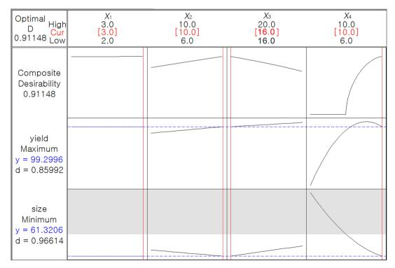
**Figure 2**. Optimum conditions of selective spray-dried nanocapsules of red ginseng extract by response surface methodology (RSM).  $X_1$ : W/O ratio;  $X_2$ : 1<sup>st</sup> emulsifier;  $X_3$ : W/O/W ratio;  $X_4$ : 2<sup>nd</sup> emulsifier;  $Y_1$ : encapsulation yield;  $Y_2$ : average particle size.
