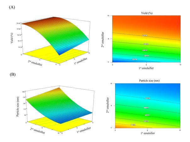
Figure 1. Response surface plots for the effects of variables on the encapsulated yield (%) (A) and the average particle size (nm) (B) of spray-dried nanocapsules of red ginseng extract.
