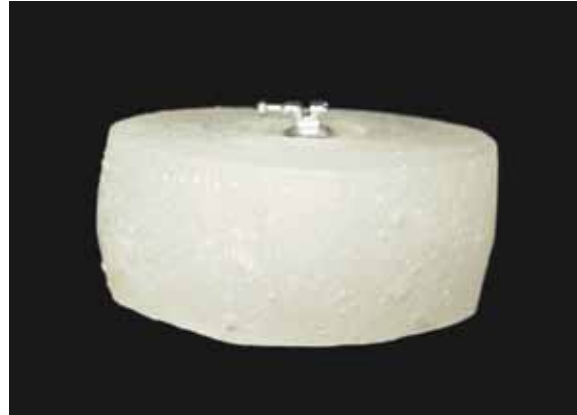
FIGURE 5 - Specimen bonded to ceramic veneer attached to acrylic resin cylinder with bracket base parallel to cylinder surface (lateral distal view of bracket).
