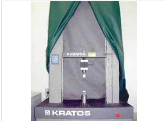
FIGURE 6 - KRATOS Universal Testing Machine, Department of Prosthodontics, Bauru School of Dentistry, University of São Paulo.
