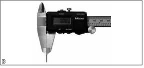
FIGURE 2 - Images showing digital caliper with A) its original tips (short) and B) the modified tips (long).
