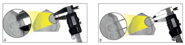
FIGURE 3 - Mesiodistal measurement of a first upper premolar using the digital caliper with A) its original tips (short) and B) the modified tips (long).
