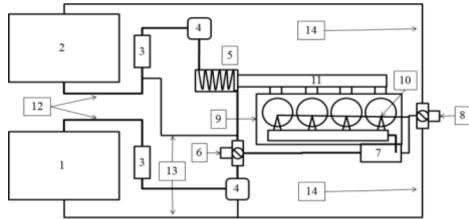
1 – Petrodiesel Tank; 2 – OV50 Tank; 3 – Feeder Electrical Bombs; 4 – Combustible Filters; 5 – Heating System; 6 – Conversion Valve of Feed; 7 – High Feeder Bomb; 8 – Conversion Valve of Feed Return; 9 – Engine; 10 – Injectors; 11 – Exhaust; 12 – Feeder Tubing; 13 – Tubing of Return of Feeder Bombs; 14 – Tubing of Return of Feed System.
