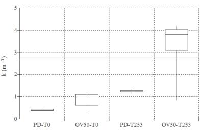
FIGURE 2. Box-plot of the medians and quartiles for the opacity to petrodiesel (PD) and the blend (OV50) at times T0 and T253 hours of work.
