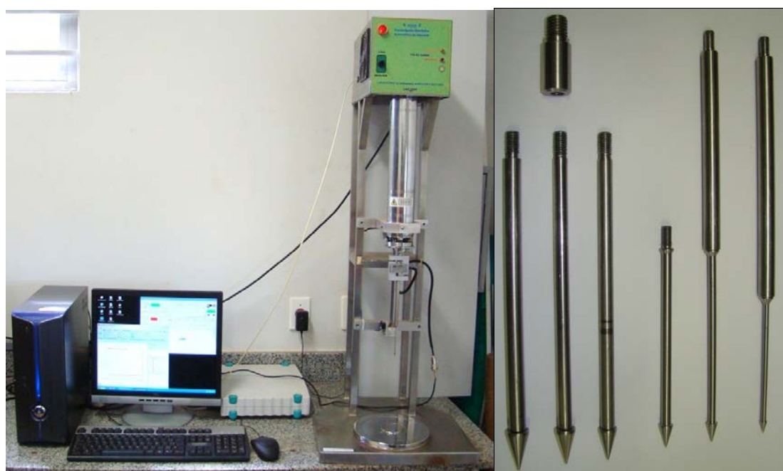
FIGURE 1. Automated bench top electronic penetrometer (ABEP) and penetration cones.
