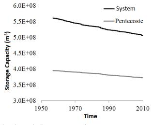
FIGURE 6. Storage capacity decay in Pentecoste weir.
