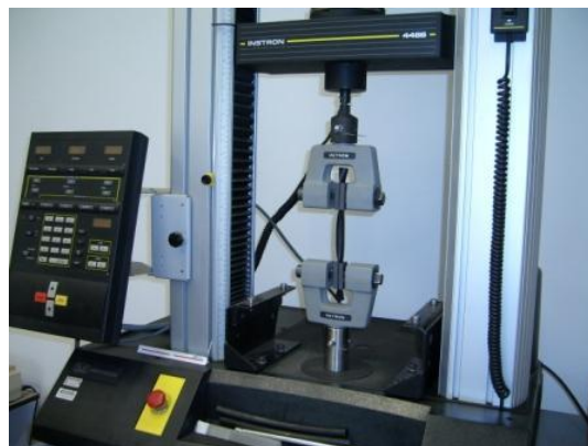
FIGURE 2. Tensile test machine used to determine modulus of elasticity of polyethylene pipes.
