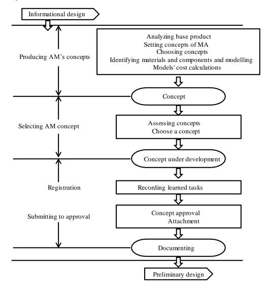
FIGURE 3. Scheme of the conceptual design phase.
