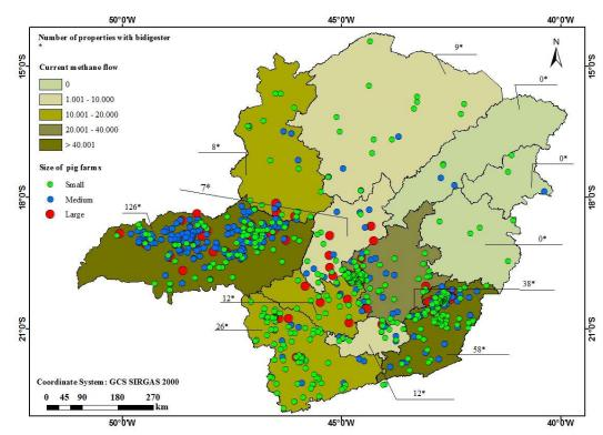
FIGURE 3. Spatial distribution of pig farms in the state of Minas Gerais by size, as well as the total methane flow grouped by mesoregion, considering pig farms with installed digesters.
