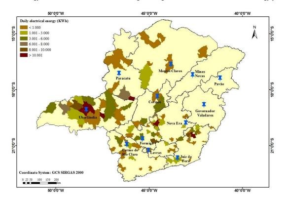
FIGURE 6. Estimation of the daily electrical energy generation available in the state of Minas Gerais from the energy utilization of biogas in pig farms.
