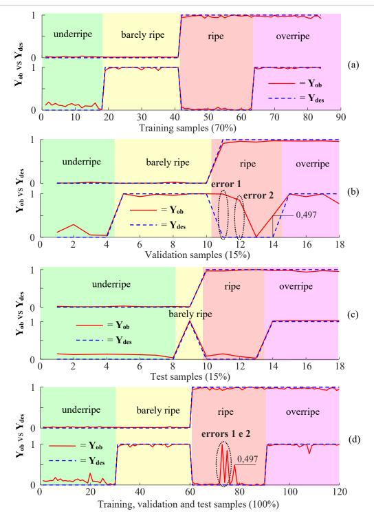
FIGURE 5. ANN performance, output obtained ( $Y_{ob}$ ) vs desired output ( $Y_{des}$ ), (a) in the training phase (70% of samples), 84 samples, (b) in the validation phase (15% of samples that were not part of the training), 18 samples, (c) in the test phase (15% of samples that were not part of the training), 18 samples, (d) in three phases (100% of samples), 120 samples.
