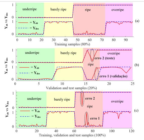
FIGURE 4. ANN performance, output obtained ( $Y_{ob}$ ) vs desired output ( $Y_{des}$ ), (a) in the training phase (80% of samples), 96 samples, (b) in the validation and test phase (20% of samples that were not part of the training), 24 samples, (c) in three phases (100% of samples), 120 samples.
