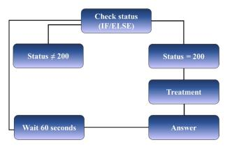
FIGURE 3. Data request and filtering tasks. Source: The Authors.
