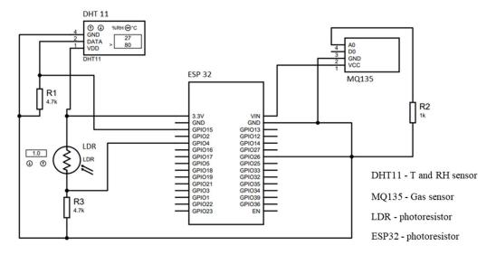
FIGURE 1. Electrical circuit of the developed board. Source: The Authors.
