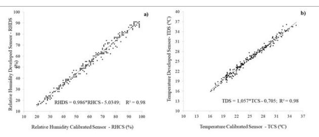
FIGURE 4. Calibration curves of the collected data, Figure 4.a) Relative Humidity Calibration Curve and Figure 4.b) Temperature Calibration Curve. Dourados/MS, 2022
