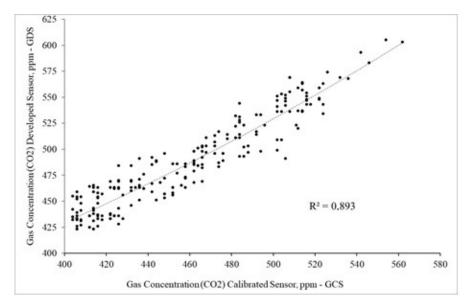
FIGURE 5. Gas concentration calibration curves. Dourados/MS, 2022.
