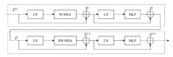
FIGURE 5. Structure of the Swin Transformer block.
