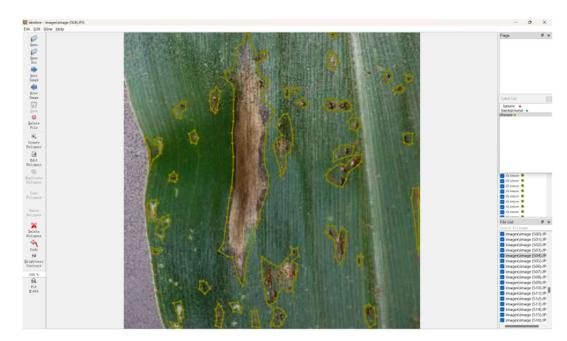
FIGURE 2. Interface used to mark the locations of maize leaf disease in an image.
