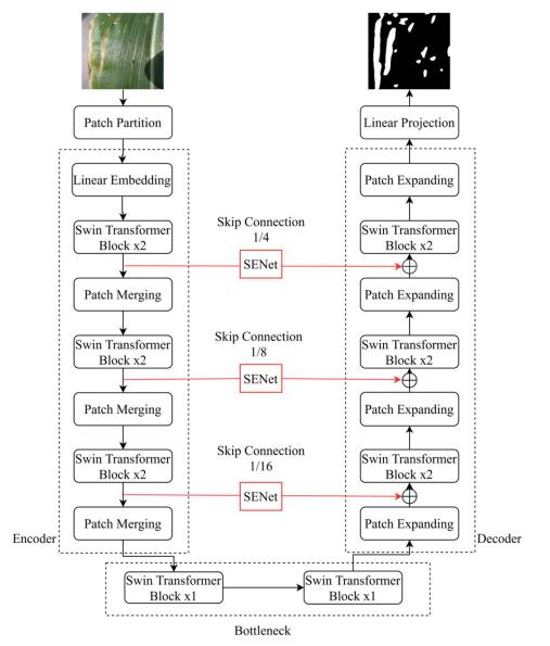
FIGURE 4. Structure of SE-Swin Unet.
