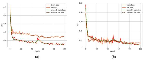
FIGURE 6. Curves showing the change in the hybrid loss functions over the training epochs: (a) CE+Dice; (b) BCE+Dice.
