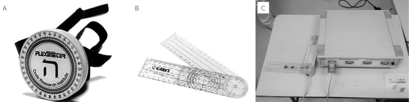
Figure 1. Instruments: (A) inclinometer; (B) goniometer; (C) electrogoniometer
