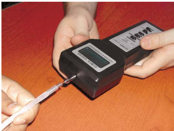
Figure 1 – Photograph of the hand-position taken by a left-handed individual being tested on an Extech™ Digital Force Gauge - model 475040. Participants were asked to hold the silicone portion and press on the tubing similar to advancing a catheter. A plastic shield (not shown) was placed between the force gauge and catheter to blind participants to their results.
