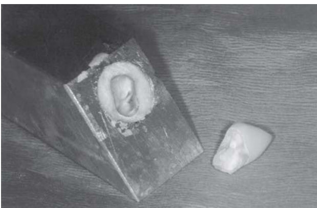
FIGURE 6- Catastrophic fracture mode in the ZI group. The line of fracture is located more than 1mm below the acrylic level
