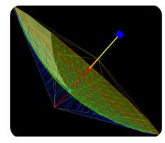
Figure 1. The space large deployable convergent membrane solar concentrator.
