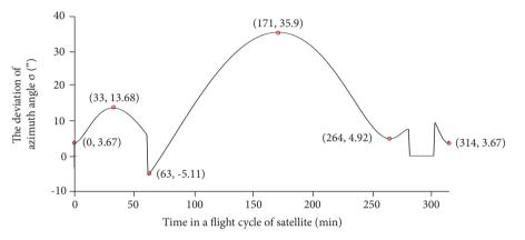
**Figure 8.** Curve of the deviation of the azimuth angle  $\sigma$  in a flight period.
