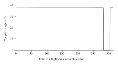
**Figure 7.** Curve of the pitch angle  $\gamma$  in a flight period.
