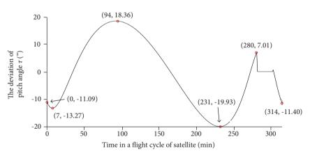
**Figure 9.** Curve of the deviation of the pitch angle  $\tau$  in a flight period.
