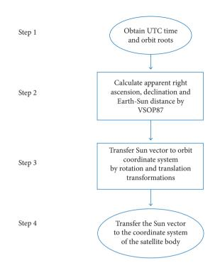
Figure 2. Procedure for the improved algorithm.
