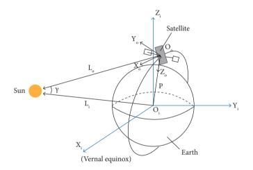
Figure 5. Deviation of sun position on the satellite caused by the size of the orbit.
