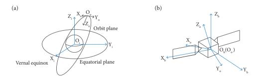
Figure 3. Correlative coordinate systems: (a) second equatorial coordinate system and orbit coordinate system; (b) orbit coordinate system and coordinate system of satellite body.
