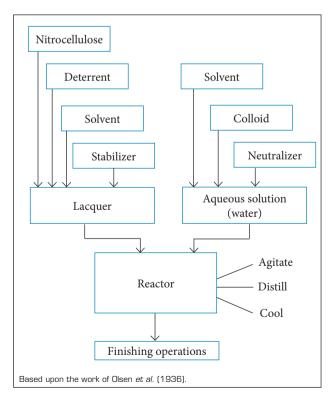
Figure 1. Spherical powder manufacturing process.
