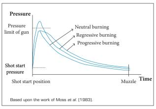
Figure 2. Pressure-time curves for different burning rates.
