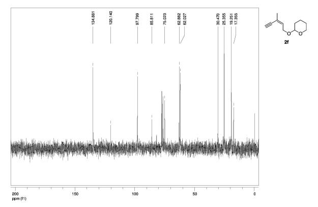
Figure S14. <sup>13</sup>C NMR of 2f (50 MHz, CDCl<sub>3</sub>).
