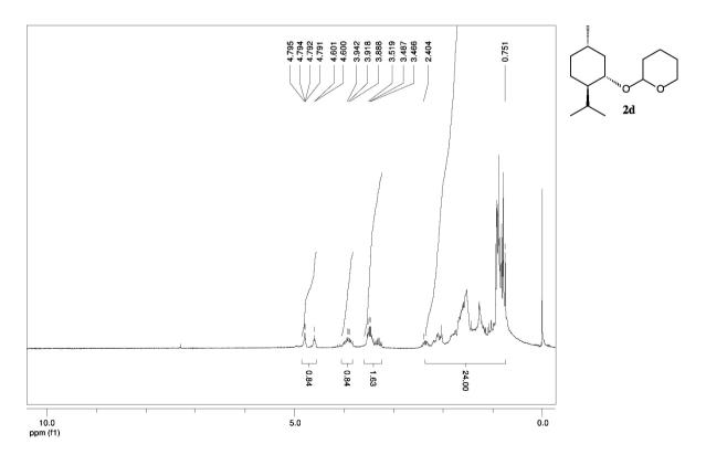
Figure S9. <sup>1</sup>H NMR of 2d (200 MHz, CDCl<sub>3</sub>).
