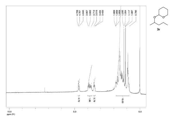
Figure S11. <sup>1</sup>H NMR of 2e (200 MHz, CDCl<sub>3</sub>).
