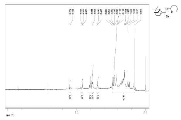
Figure S17. <sup>1</sup>H NMR of 2h (200 MHz, CDCl<sub>3</sub>).
