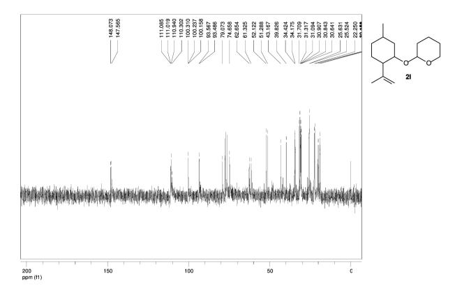
**Figure S28.** <sup>13</sup>C NMR of **2l** (50 MHz, CDCl<sub>3</sub>).
