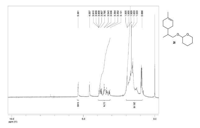
Figure S21. <sup>1</sup>H NMR of 2i (200 MHz, CDCl<sub>3</sub>).
