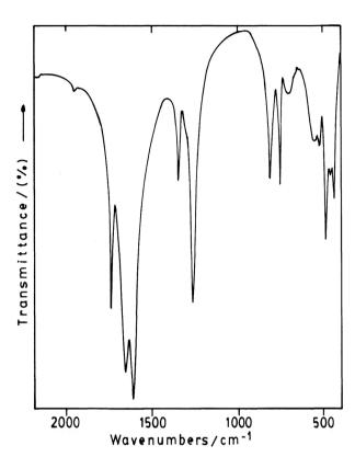
**Figure 4.** FT-Infrared spectrum of  $Fe_2(C_2O_4)_3$ - $4H_2O$  in the spectral range between 2000 and 400 cm $^{-1}$ .
