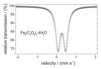
**Figure 5.** 298 K <sup>57</sup>Fe-Mössbauer spectrum of Fe<sub>2</sub>(C<sub>2</sub>O<sub>4</sub>)<sub>3</sub>·4H<sub>2</sub>O.
