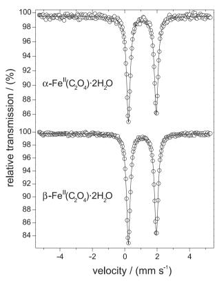
**Figure 3.** 298 K <sup>57</sup>Fe-Mössbauer spectra of the two modifications of  $Fe(C_2O_3) \cdot 2H_2O$ .
