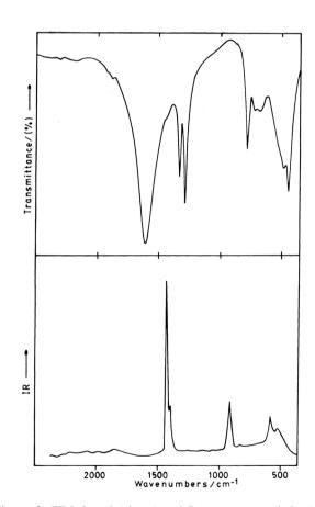
**Figure 2.** FT-Infrared (above) and Raman spectra (below) of  $\alpha$ -Fe(C<sub>2</sub>O<sub>4</sub>)•2H<sub>2</sub>O in the spectral range between 2000 and 400 cm<sup>-1</sup>.
