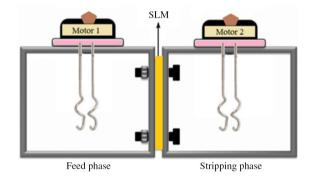
Figure 1. Schematic presentation of liquid membrane permeator cell.
