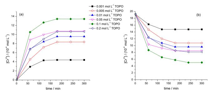
Figure 2. Variation in  $Cr^{VI}$  ion concentration with time in the (a) strip and (b) feed solutions at various concentrations of TOPO (initial  $[Cr^{VI}] = 19.2 \times 10^4 \text{ mol } L^{-1}$ ,  $[H_2O_2] = 0.5 \text{ mol } L^{-1}$ ,  $[DPC] = 0.001 \text{ mol } L^{-1}$ ,  $[H_2SO_4] = 1 \text{ mol } L^{-1}$ ,  $[TOPO] = 0.001 \text{ -0.2 mol } L^{-1}$ ).
