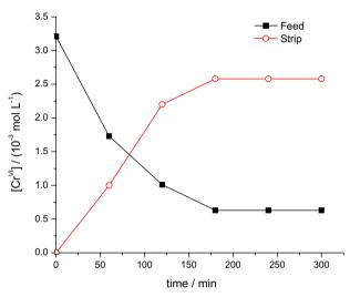
**Figure 11.** Variation in  $Cr^{VI}$  ion concentration in the feed and strip solution *vs.* time (paint industry waste solution in feed) (initial  $[Cr^{VI}] = 3.21 \times 10^{-3} \text{ mol } L^{-1}, [H_2O_2] = 1.5 \text{ mol } L^{-1}, [DPC] = 0.001 \text{ mol } L^{-1}, [H_3O_4] = 1.5 \text{ mol } L^{-1}, [TOPO] = 0.1 \text{ mol } L^{-1}).$
