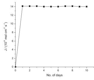
Figure 10. Stability of SLM, flux vs. time (initial  $[Cr^{VI}] = 19.2 \times 10^{-4} \text{ mol } L^{-1}$ ,  $[H_2O_2] = 1.5 \text{ mol } L^{-1}$ ,  $[DPC] = 0.001 \text{ mol } L^{-1}$ ,  $[H_2SO_4] = 1.5 \text{ mol } L^{-1}$ ,  $[TOPO] = 0.1 \text{ mol } L^{-1}$ ).
