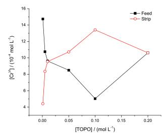
**Figure 3.** Variation in  $Cr^{VI}$  ion concentration in the feed and strip solution at various concentrations of TOPO (initial  $[Cr^{VI}] = 19.2 \times 10^4$  mol L<sup>-1</sup>,  $[H_2O_2] = 0.5$  mol L<sup>-1</sup>, [DPC] = 0.001 mol L<sup>-1</sup>,  $[H_2SO_4] = 1$  mol L<sup>-1</sup>, [TOPO] = 0.001-0.2 mol L<sup>-1</sup>).
