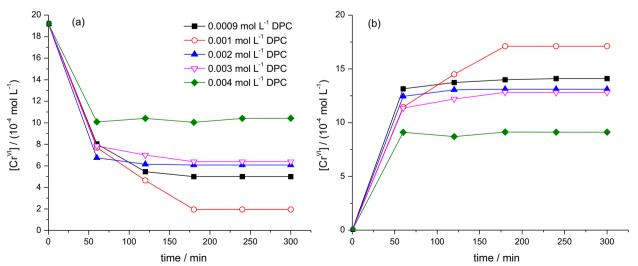
**Figure 6.** Variation in  $Cr^{VI}$  ion concentration with time in the (a) feed and (b) strip solutions at various concentrations of diphenylcarbazide (DPC) (initial  $[Cr^{VI}] = 19.2 \times 10^4 \text{ mol } L^{-1}$ ,  $[H_2O_2] = 0.5 \text{ mol } L^{-1}$ ,  $[DPC] = 0.0005 - 0.004 \text{ mol } L^{-1}$ ,  $[H_2SO_4] = 1 \text{ mol } L^{-1}$ ,  $[TOPO] = 0.1 \text{ mol } L^{-1}$ ).
