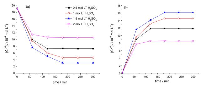
Figure 8. Variation in  $Cr^{VI}$  ion concentration with time in the (a) feed and (b) strip solutions at various concentrations of  $H_2SO_4$  (initial  $[Cr^{VI}] = 19.2 \times 10^4 \text{ mol } L^{-1}$ ,  $[H_2O_2] = 0.5 \text{ mol } L^{-1}$ ,  $[DPC] = 0.001 \text{ mol } L^{-1}$ ,  $[H_2SO_4] = 0.5-2 \text{ mol } L^{-1}$ ,  $[TOPO] = 0.1 \text{ mol } L^{-1}$ ).
