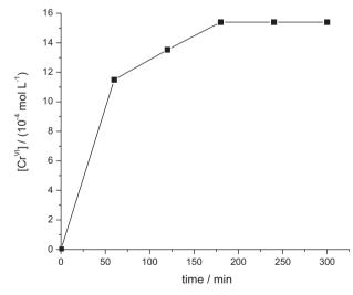
**Figure 9.** Variation in  $Cr^{VI}$  ion concentration with time (initial  $[Cr^{VI}] = 19.2 \times 10^4 \text{ mol } L^{-1}, [H_2O_2] = 1.5 \text{ mol } L^{-1}, [DPC] = 0.001 \text{ mol } L^{-1}, [H_2SO_4] = 1.5 \text{ mol } L^{-1}, [TOPO] = 0.1 \text{ mol } L^{-1}).$
