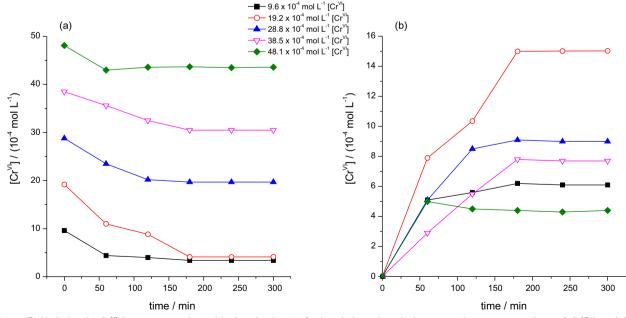
**Figure 7.** Variation in  $Cr^{VI}$  ion concentration with time in the (a) feed and (b) strip solutions at various concentrations of  $Cr^{VI}$  ion (initial  $[Cr^{VI}] = 9.6 \times 10^4 - 48.1 \times 10^4$  mol L<sup>-1</sup>,  $[H_2O_2] = 0.5$  mol L<sup>-1</sup>, [DPC] = 0.001 mol L<sup>-1</sup>,  $[H_2SO_4] = 1.5$  mol L<sup>-1</sup>, [TOPO] = 0.1 mol L<sup>-1</sup>).
