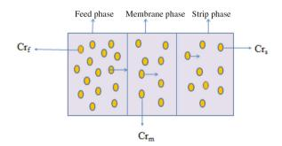
Figure 4. Mass transfer diagram of chromium ions.
